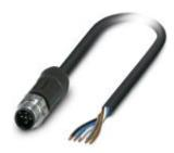
Sensor/actuator cable, 5-position, PE-X halogen-free, black-gray RAL 7021, Plug straight M12, A-coded, on free cable end, cable length: 5 m, for outdoor applications, with high-grade steel knurl
