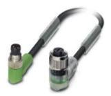
Sensor/actuator cable, 3-position, PUR halogen-free, black-gray RAL 7021, Plug angled M8, on Socket angled M12, A-coded, with 2 LEDs, cable length: 0.3 m
