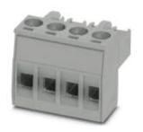
Plug component, Nominal current: 16 A, Rated voltage (III/2): 320 V, Number of positions: 4, Pitch: 5 mm, Connection method: Screw connection
