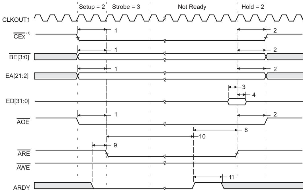
1.  $\overline{\text{CEx}}$  stays active for 7 – the value of Read Hold cycles after the last access (DMA transfer or CPU access). For example, if read HOLD = 1, then  $\overline{\text{CEx}}$  stays active for six more cycles. This does not affect performance, it merely reflects the overhead of the EMIF.
