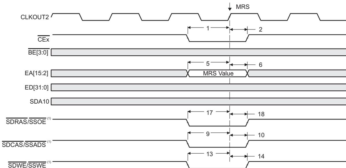
1. SDCAS/SSADS, SDRAS/SSOE, and SDWE/SSWE operate as SDCAS, SDRAS, and SDWE, respectively, during SDRAM accesses.
