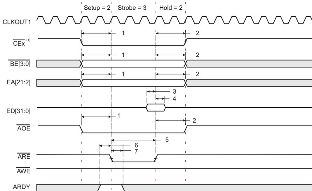
1.  $\overline{\text{CEx}}$  stays active for 7 – the value of Read Hold cycles after the last access (DMA transfer or CPU access). For example, if read HOLD = 1, then  $\overline{\text{CEx}}$  stays active for six more cycles. This does not affect performance, it merely reflects the overhead of the EMIF.
