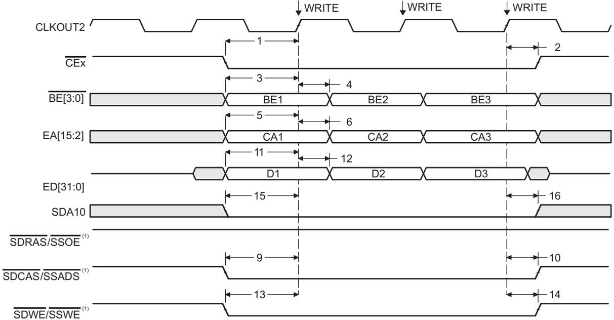
1.  $\overline{\text{SDCAS}}/\overline{\text{SSADS}}$ ,  $\overline{\text{SDRAS}}/\overline{\text{SSOE}}$ , and  $\overline{\text{SDWE}}/\overline{\text{SSWE}}$  operate as  $\overline{\text{SDCAS}}$ ,  $\overline{\text{SDRAS}}$ , and  $\overline{\text{SDWE}}$ , respectively, during SDRAM accesses.
