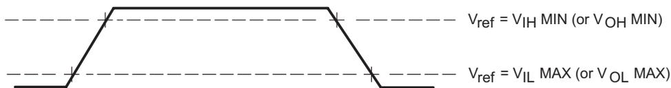
Figure 3. Rise and Fall Transition Time Voltage Reference Levels
