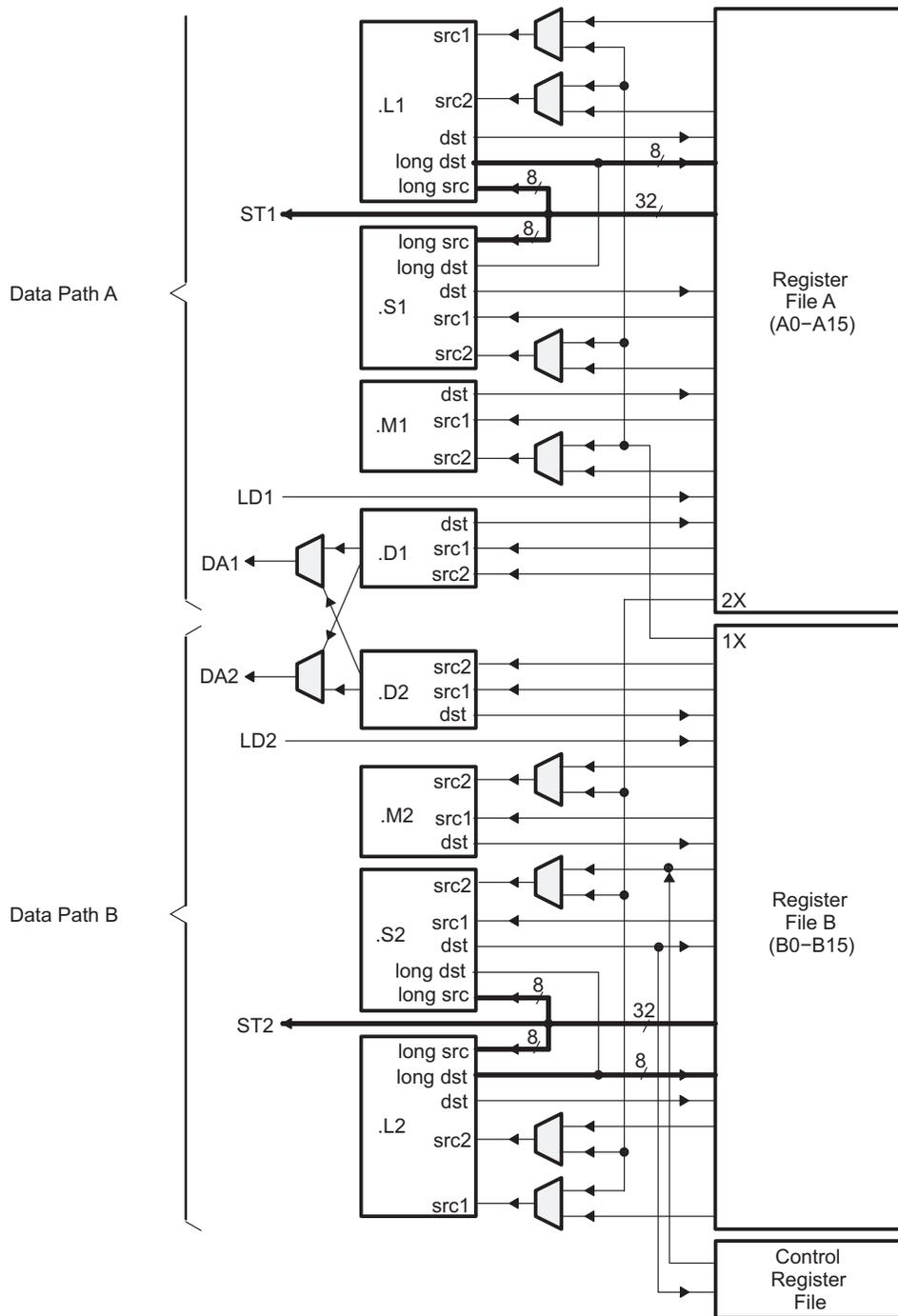
Figure 53. SMJ320C62x CPU (DSP Core) Data Paths
