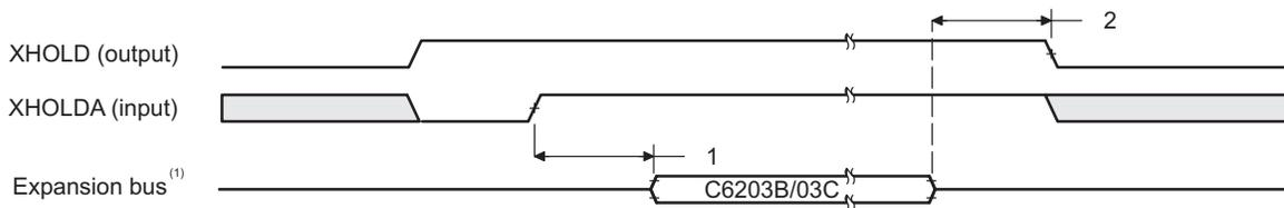
1. Expansion bus consists of  $\overline{XBE}[3:0]/XA[5:2]$ ,  $\overline{XAS}$ ,  $XW/R$ , and  $XBLAST$ .
