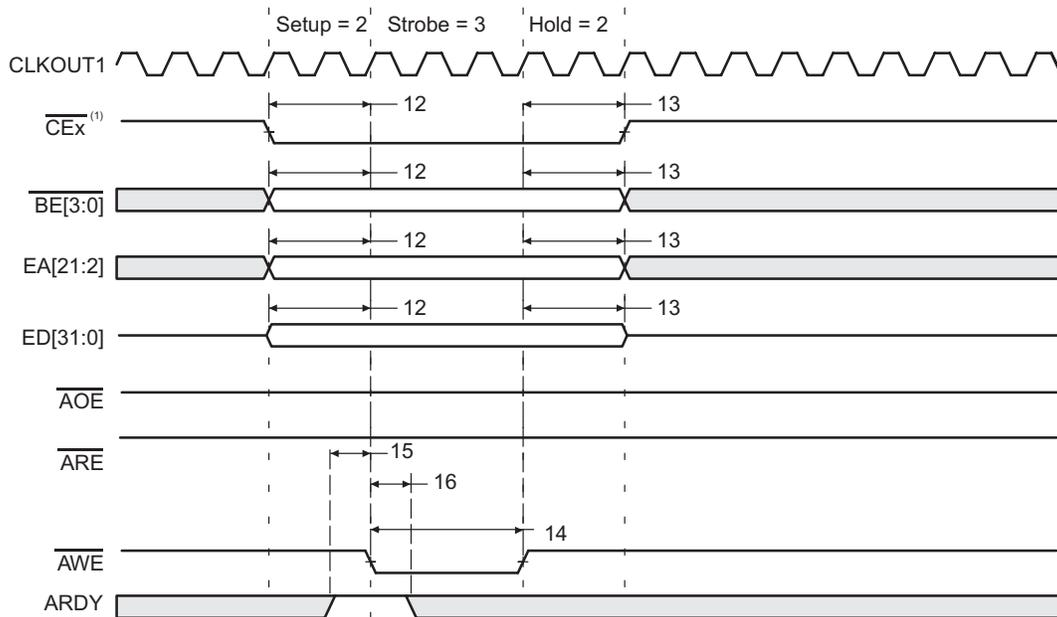
1. If no write accesses are scheduled for the next cycle and write hold is set to 1 or greater, then  $\overline{\text{CEx}}$  stays active for three cycles after the value of the programmed hold period. If write hold is set to 0, then  $\overline{\text{CEx}}$  stays active for four more cycles. This does not affect performance, it merely reflects the overhead of the EMIF.
