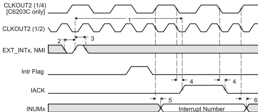
**Figure 23. Interrupt Timing**
