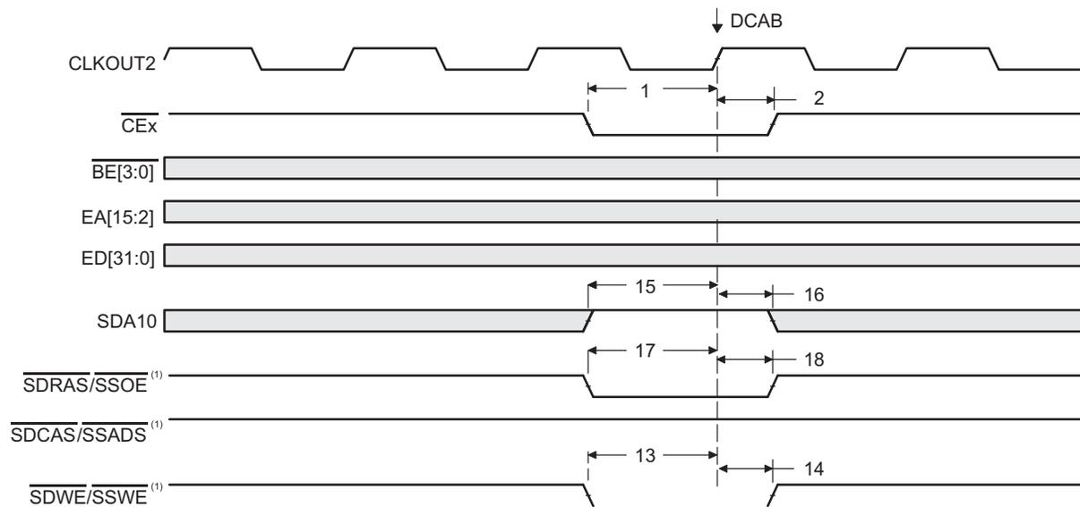
1. SDCAS/SSADS, SDRAS/SSOE, and SDWE/SSWE operate as SDCAS, SDRAS, and SDWE, respectively, during SDRAM accesses.
