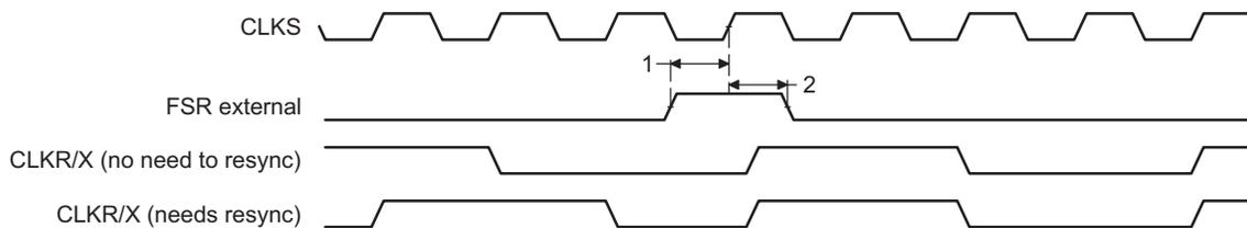
**Figure 41. FSR Timing When GSYNC = 1**
