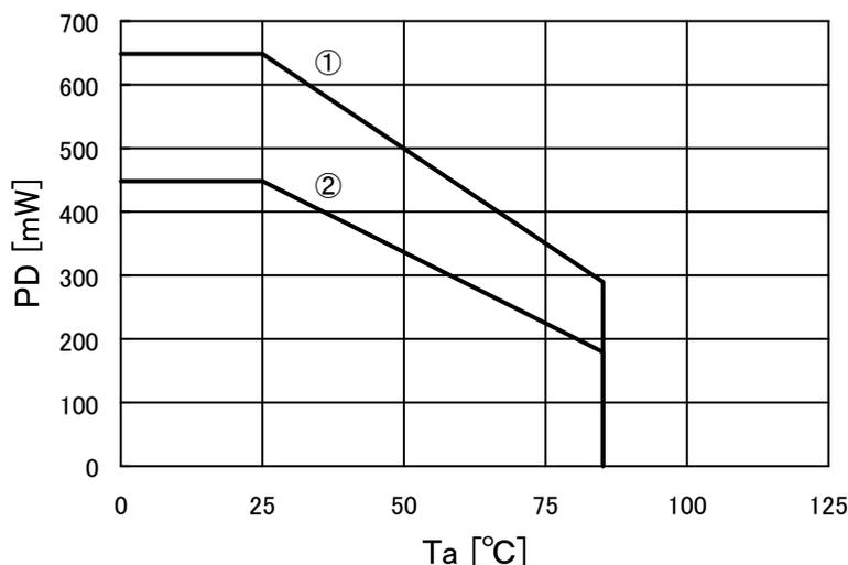
Mounted on a 70x70x1.6mm FR4 glass epoxy board (copper foil area 3% or below)
