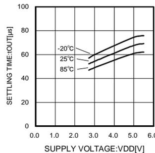
Fig.16 Settling time
