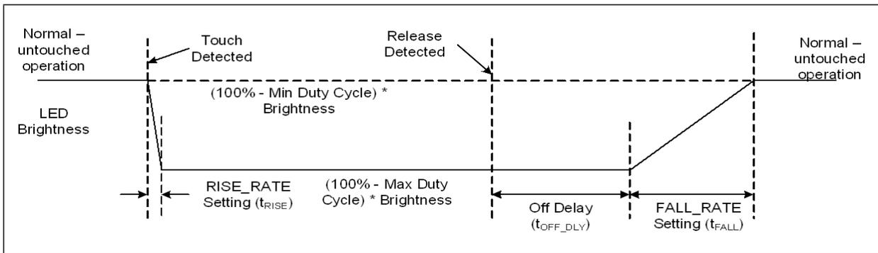
**FIGURE 6-8: Direct Behavior for Inverted Polarity**
