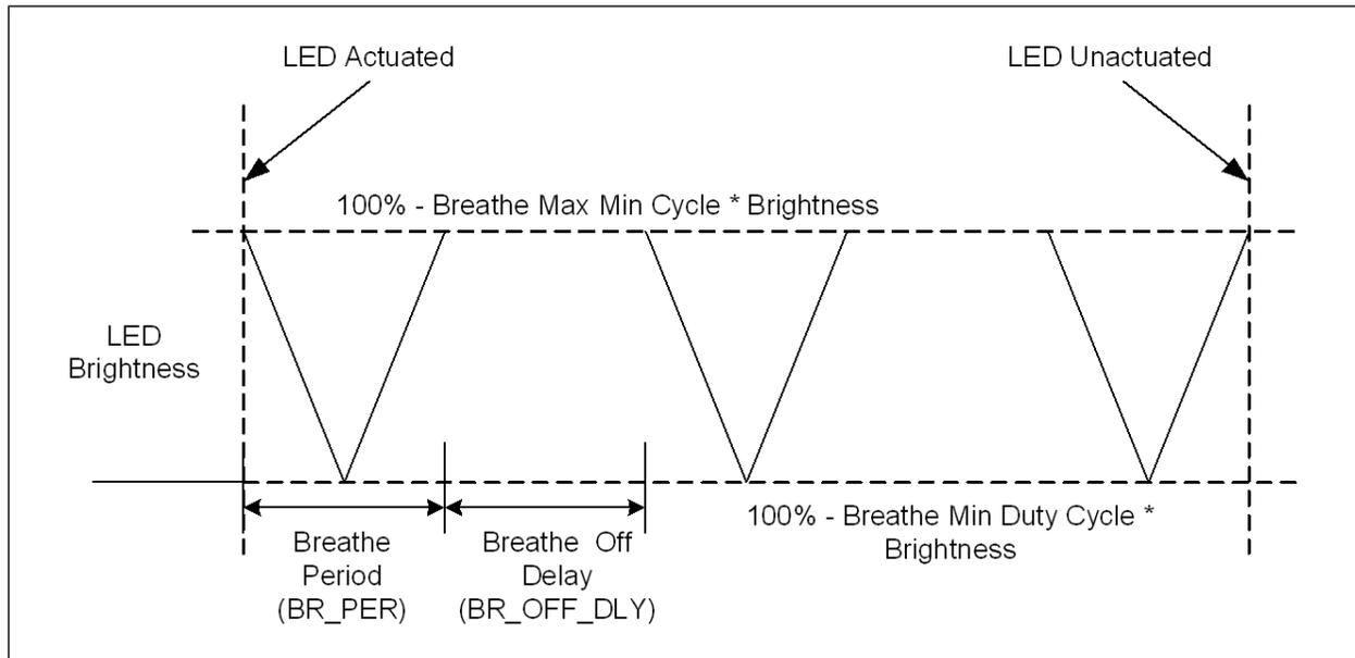
**FIGURE 6-6:** *Breathe Behavior with Inverted Polarity*
