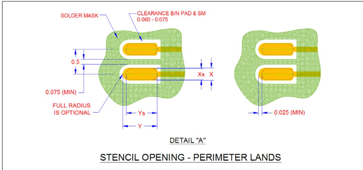
**FIGURE 7-5:** CAP1188 PCB Detail B - 24-Pin QFN 4mm x 4mm
