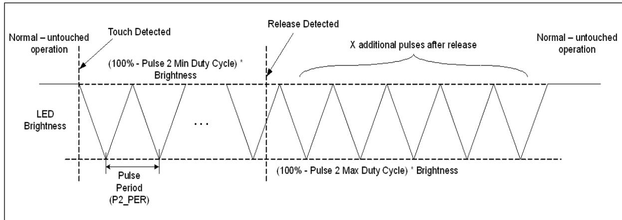
**FIGURE 6-4: Pulse 2 Behavior with Inverted Polarity**
