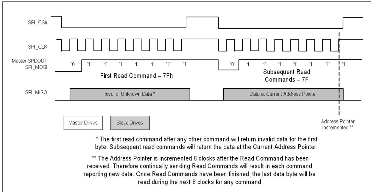
**FIGURE 4-8:** SPI Read Command - Normal Mode - Full
