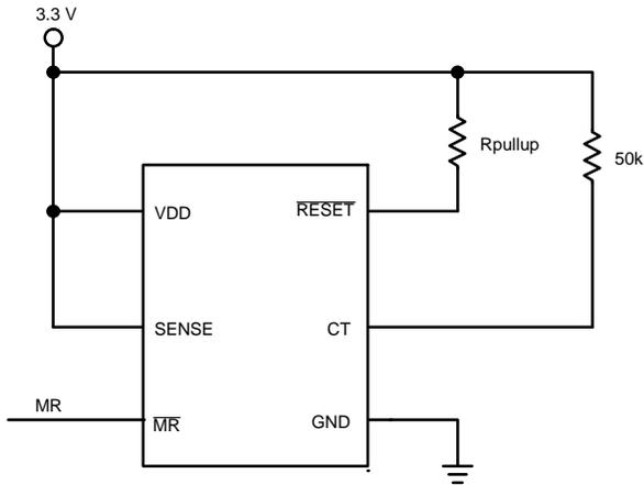
**Figure 14. Delay Time Fixed to 300 ms when CT Connected to V<sub>DD</sub> by Resistor**
