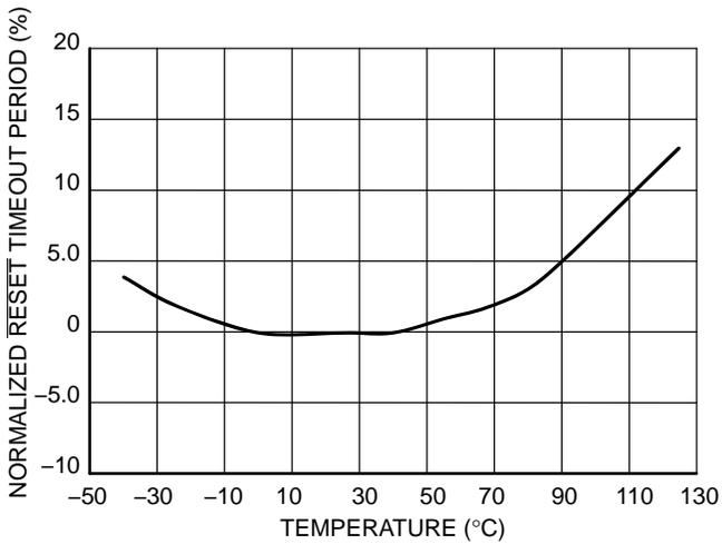
Figure 8. Normalized RESET Timeout Period vs. Temperature
