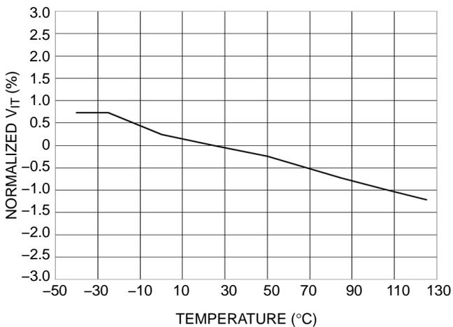
Figure 10. Normalized Sense Threshold Voltage ( $V_{IT}$ ) vs. Temperature
