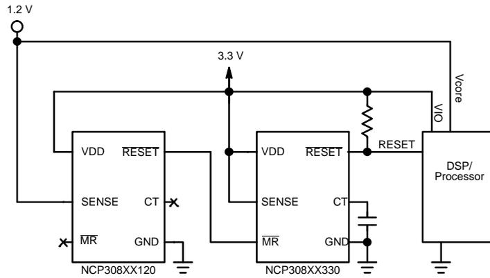
**Figure 13. Using  $\overline{MR}$  to Monitor Multiple System Voltages**
