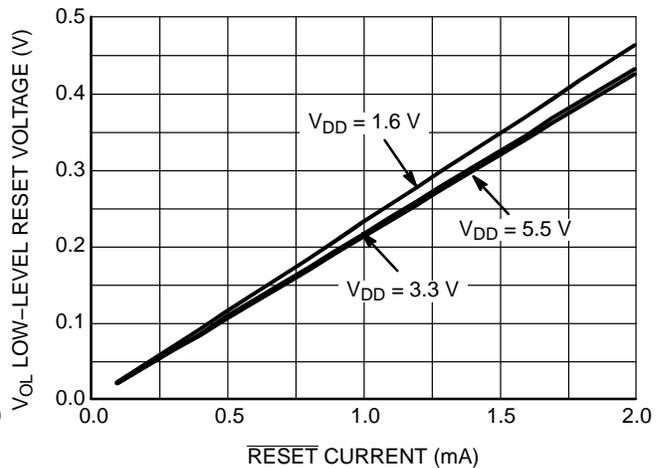
Figure 11. Low-Level RESET Voltage vs. RESET Current
