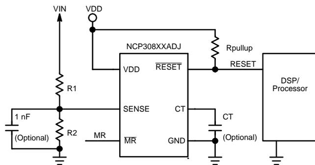
Figure 1. Typical Application Circuit for Adjustable Versions
