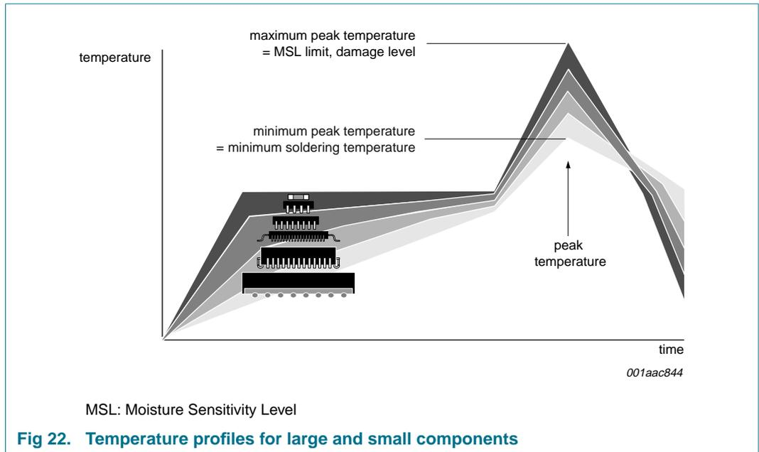
Fig 22. Temperature profiles for large and small components
