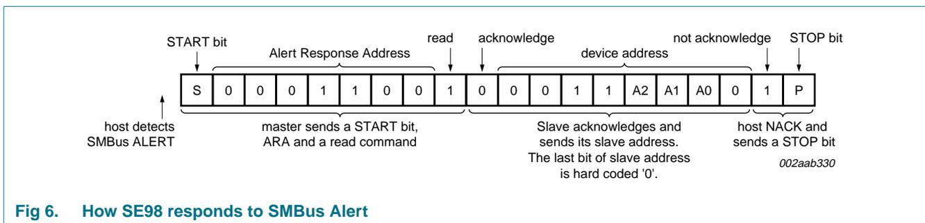
**Fig 6. How SE98 responds to SMBus Alert**
