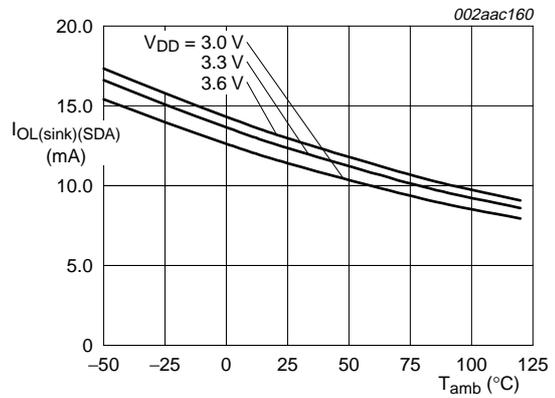
Fig 17. EVENT sink current at 0.6 V versus temperature
