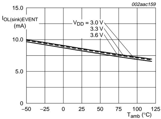
Fig 16. EVENT sink current at 0.4 V versus temperature
