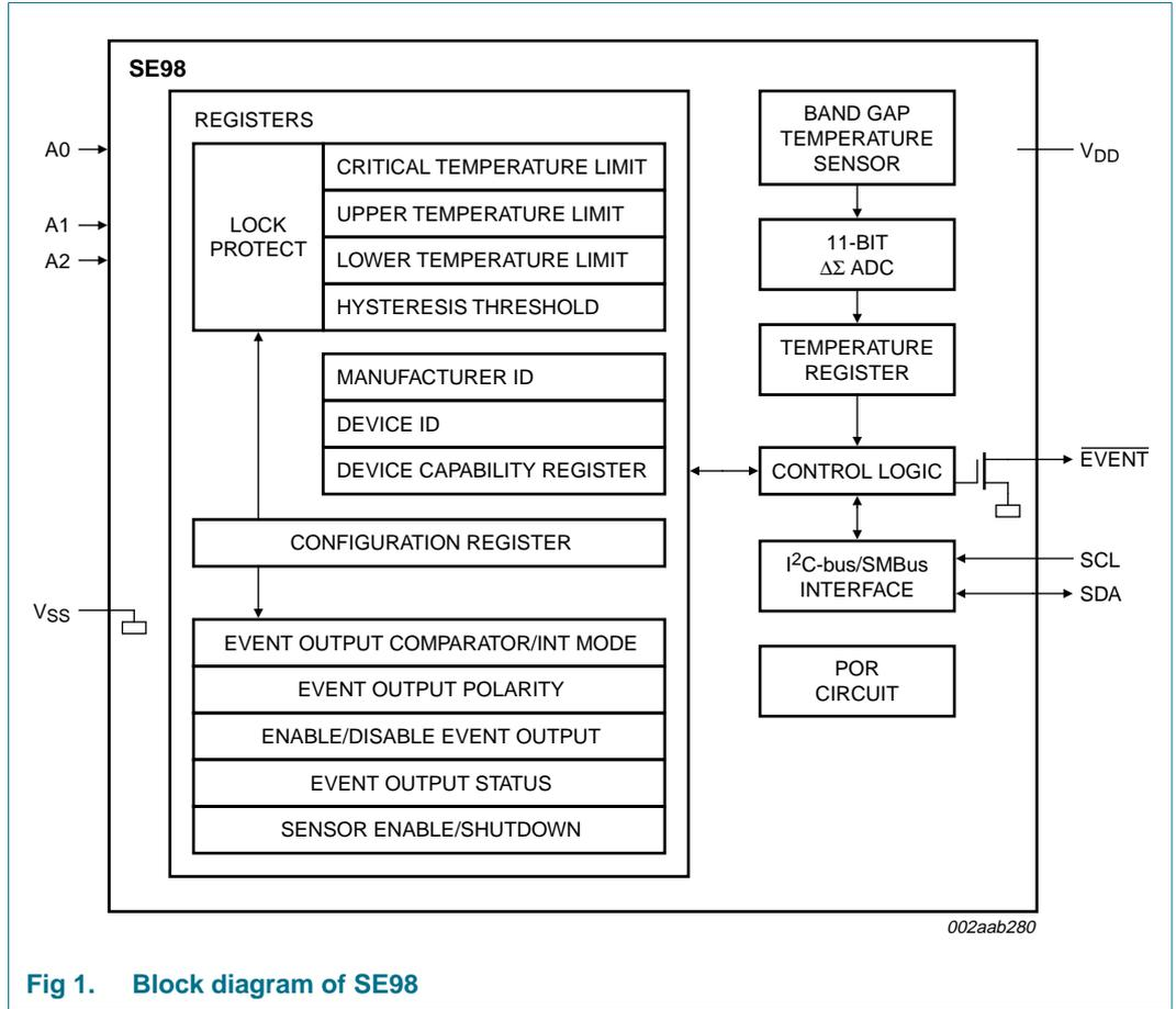
Fig 1. Block diagram of SE98
