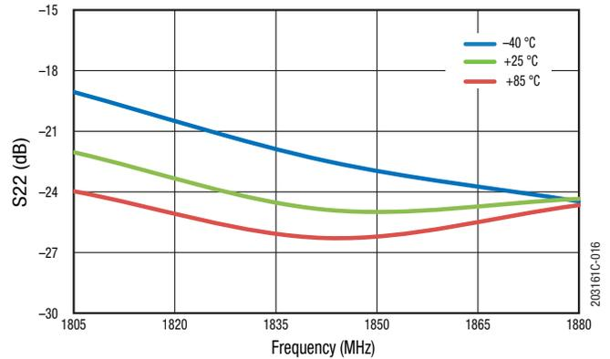
**Figure 16. Output Return Loss vs Frequency Across Temperature (Small Signal, P<sub>IN</sub> = -20 dBm)**
