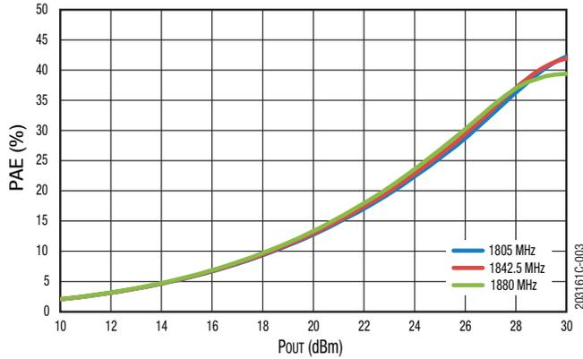
**Figure 3. PAE vs Pout Across Frequency @ 5 V, 25 °C**
