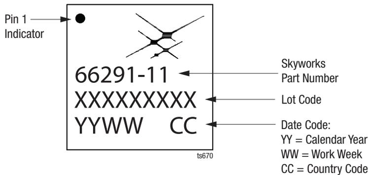
Figure 21. Typical Part Marking for the SKY66291-11
