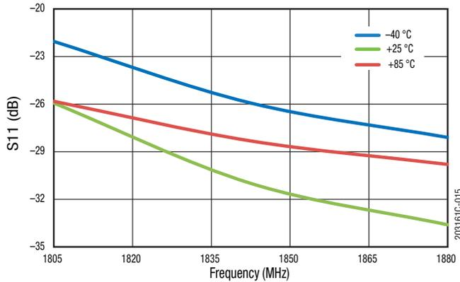
**Figure 15. Input Return Loss vs Frequency Across Temperature (Small Signal, P<sub>IN</sub> = -20 dBm)**
