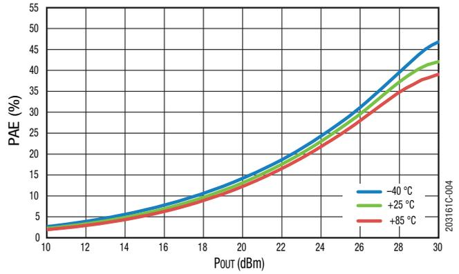
**Figure 4. PAE vs. Pout Across Temperature @ 1842.5 MHz, 5 V**
