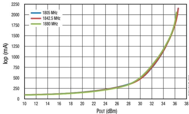
Figure 9. Operating Current vs Pout Across Frequency
