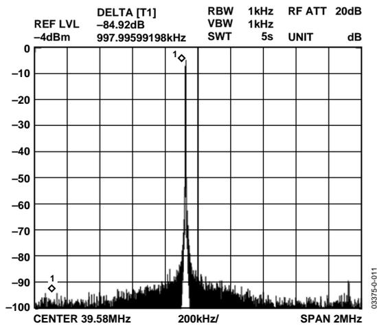
Figure 12.  $F_{OUT} = 39.9$  MHz,  $F_{CLK} = 400$  MSPS, NBSFDR,  $\pm 1$  MHz
