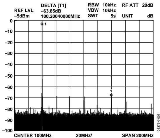
Figure 6.  $F_{OUT} = 40\text{ MHz}$ ,  $F_{CLK} = 400\text{ MSPS}$ , WBSFDR
