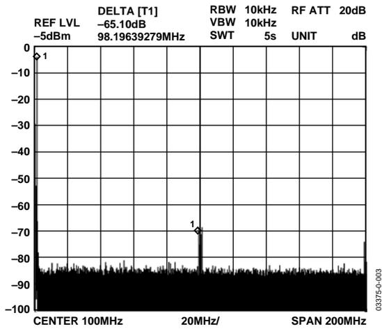
Figure 4.  $F_{OUT} = 1\text{ MHz}$ ,  $F_{CLK} = 400\text{ MSPS}$ , WBSFDR
