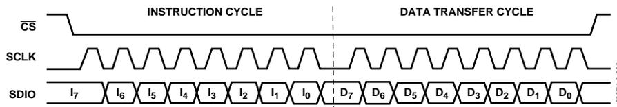
Figure 21. Serial Port Write Timing—Clock Stall Low
