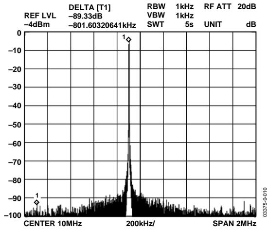
Figure 11.  $F_{OUT} = 10$  MHz,  $F_{CLK} = 400$  MSPS, NBSFDR,  $\pm 1$  MHz
