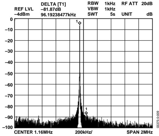
Figure 10.  $F_{OUT} = 1.1$  MHz,  $F_{CLK} = 400$  MSPS, NBSFDR,  $\pm 1$  MHz
