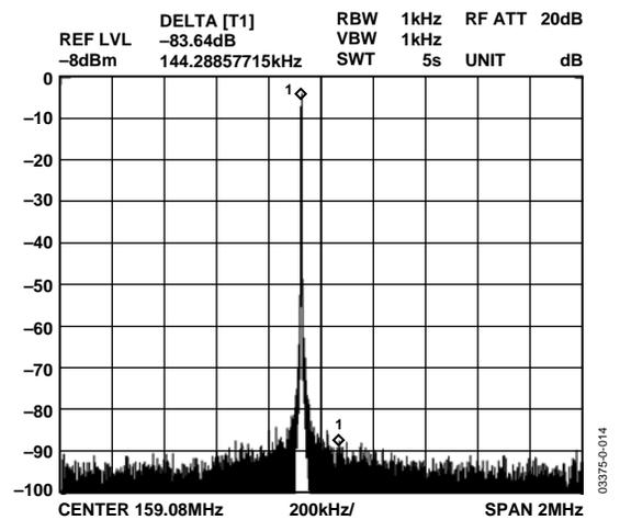
Figure 15.  $F_{OUT} = 160$  MHz,  $F_{CLK} = 400$  MSPS, NBSFDR,  $\pm 1$  MHz
