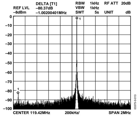
Figure 14.  $F_{OUT} = 120.2$  MHz,  $F_{CLK} = 400$  MSPS, NBSFDR,  $\pm 1$  MHz
