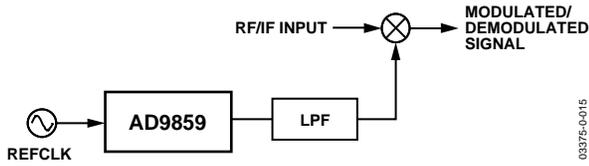
Figure 25. Synchronized LO for Up Conversion/Down Conversion
