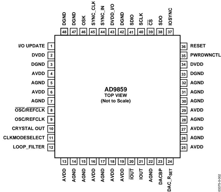
Figure 3. 48-Lead TQFP/EP
