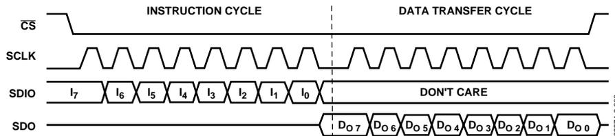
Figure 22. 3-Wire Serial Port Read Timing—Clock Stall Low
