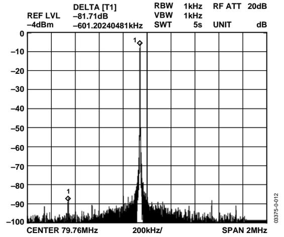
Figure 13.  $F_{OUT} = 80.3$  MHz,  $F_{CLK} = 400$  MSPS, NBSFDR,  $\pm 1$  MHz
