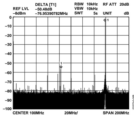
Figure 9.  $F_{OUT} = 160\text{ MHz}$ ,  $F_{CLK} = 400\text{ MSPS}$ , WBSFDR
