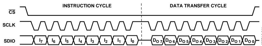
Figure 24. 2-Wire Serial Port Read Timing—Clock Stall High
