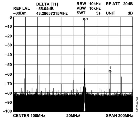
Figure 8  $F_{OUT} = 120\text{ MHz}$ ,  $F_{CLK} = 400\text{ MSPS}$ , WBSFDR
