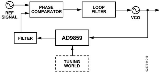
Figure 26. Digitally Programmable Divide-by-N Function in PLL
