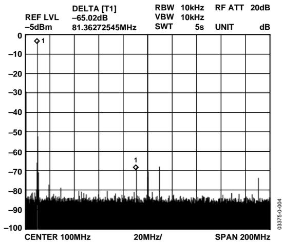
Figure 5.  $F_{OUT} = 10\text{ MHz}$ ,  $F_{CLK} = 400\text{ MSPS}$ , WBSFDR
