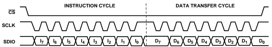
Figure 23. Serial Port Write Timing—Clock Stall High
