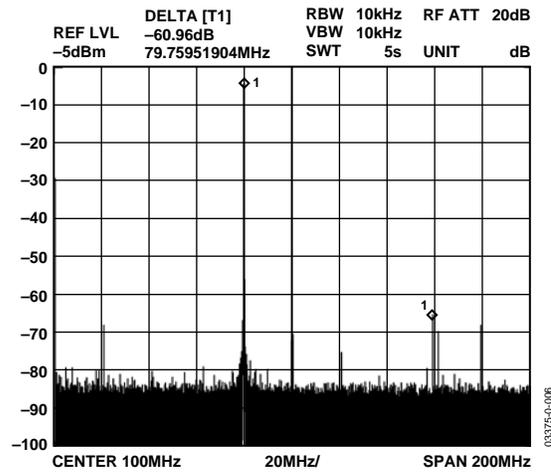
Figure 7.  $F_{OUT} = 80\text{ MHz}$ ,  $F_{CLK} = 400\text{ MSPS}$ , WBSFDR
