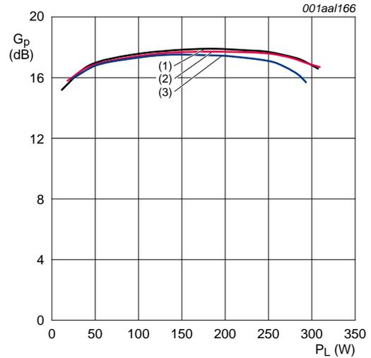
$V_{DS} = 50 \text{ V}$ ;  $t_p = 300 \text{ } \mu\text{s}$ ;  $\delta = 10 \%$ ;  $I_{Dq} = 100 \text{ mA}$ .
