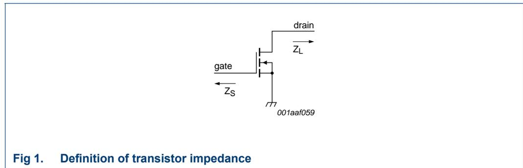
**Fig 1. Definition of transistor impedance**
