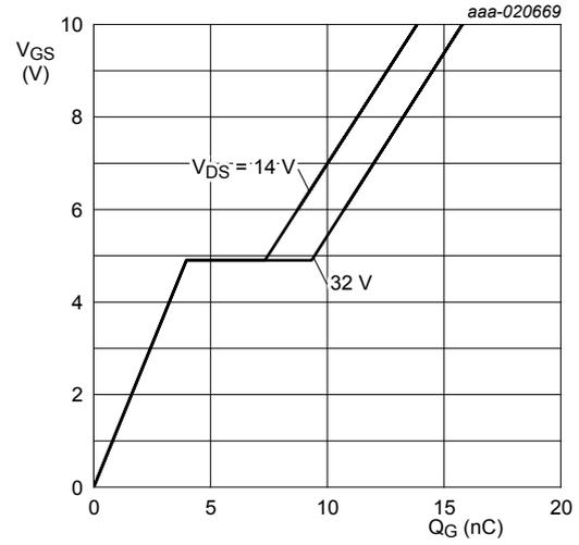
$T_j = 25^{\circ}\text{C}; I_D = 15\text{ A}$
