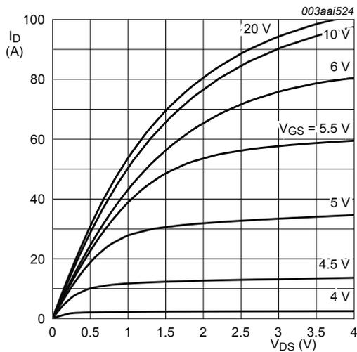
$T_j = 25\text{ °C}; t_p = 300\text{ }μs$
