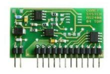
Binary input for potential-less contacts. Maximum resistance of closed contact: 1000 ohms. Minimum duration for recording: 200ms.
