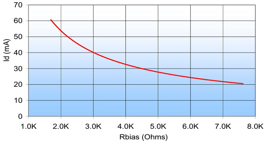
**Fig 4.**  $I_d$  varies as a function of  $R_{bias}$ . The  $I_d$  current range is defined based upon the specific  $R_{bias}$  value noted in the Application Circuit (Fig 3).  $R_{bias}$  may be adjusted to optimize  $I_d$  for a customers' application. RF performance will vary accordingly.
