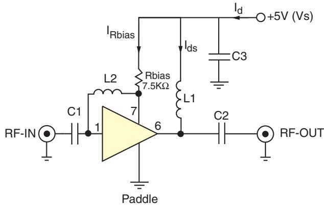
**Fig 3.** Recommended Application Circuit
