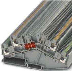
Disconnect terminal block, double level with angled contour and two disconnect points, Connection type: Push-in connection, Cross section: 0.14 mm<sup>2</sup> - 4 mm<sup>2</sup>, AWG: 26 - 12, Nominal current: 20 A, Nominal voltage: 400 V, Length: 127.5 mm, Width: 5.2 mm, Color: blue, Assembly: NS 35/7,5, NS 35/15
