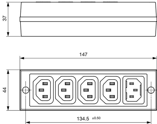
Mounting holes for 3 mm screws
