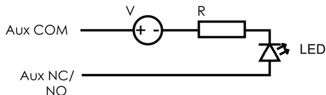
In case the contactor is stuck, the Aux COM and Aux NO wires will be short, hence the circuit is closed and the LED will be on. The AUX COM and AUX NC wires will be have the opposite way: the LED will be off when the contactor is stuck.
