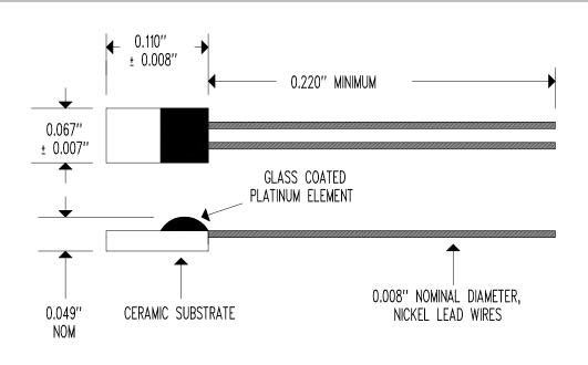
RTD ELEMENT RESISTANCE @ 0°C = 100  $\Omega$  ± 0.24% RTD ELEMENT ACCURACY @ 0°C = ± 0.60°C
