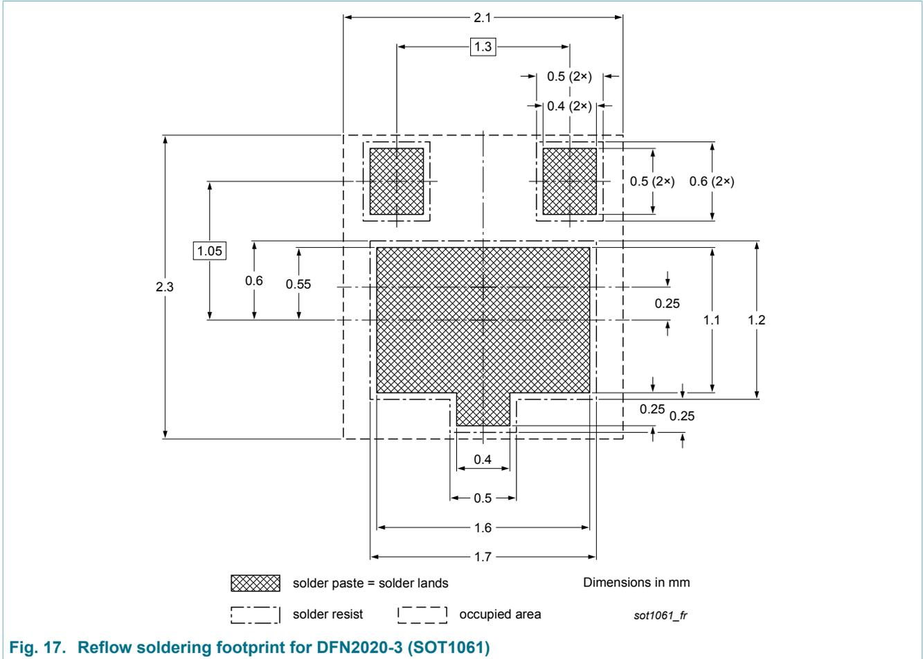
Fig. 17. Reflow soldering footprint for DFN2020-3 (SOT1061)
