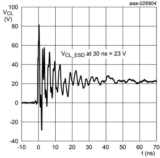
Fig. 13. Clamped +8 kV pulse waveform (IEC 61000-4-2 network)
