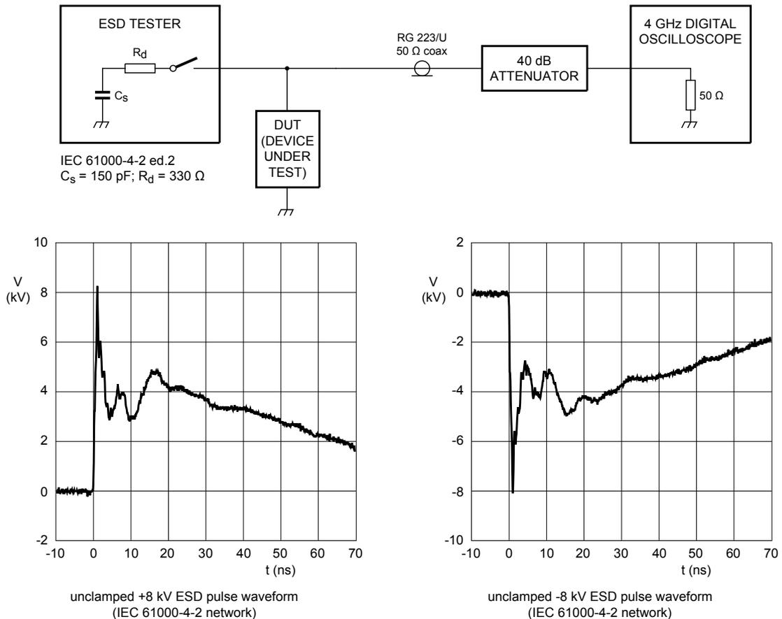
Fig. 12. ESD clamping test setup and waveforms
