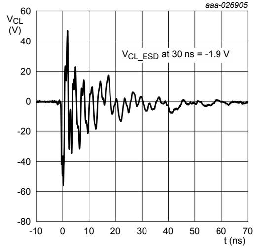
Fig. 14. Clamped -8 kV pulse waveform (IEC 61000-4-2 network)
