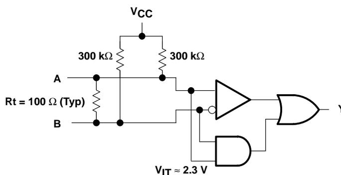
Figure 11. Open-Circuit Fail Safe of the LVDS Receiver
