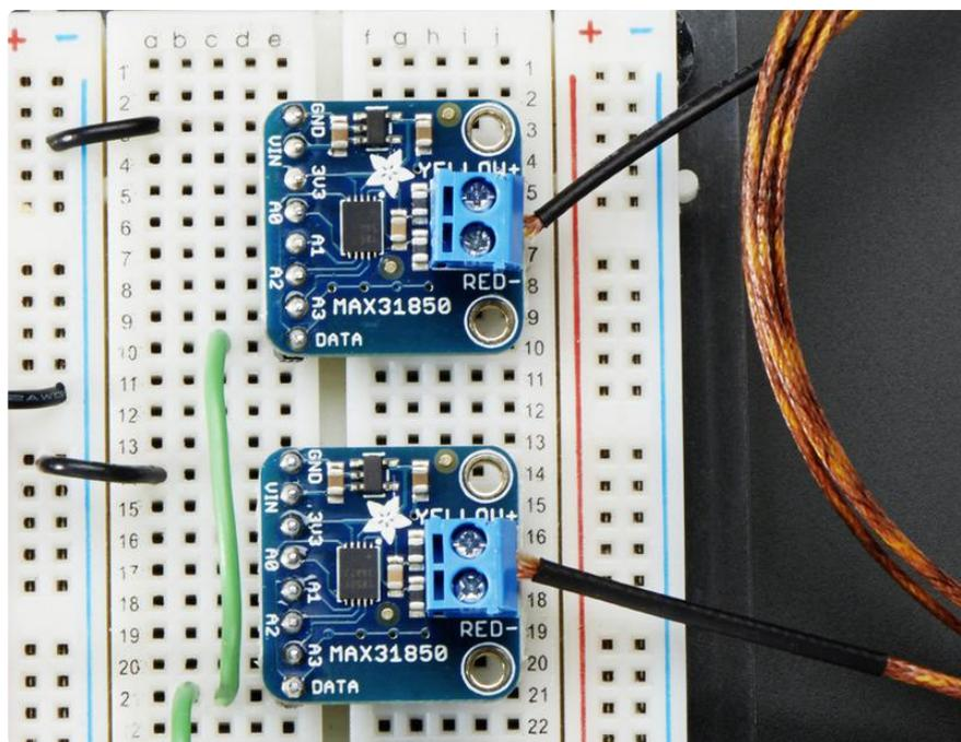
The MAX31850K data format is very similar to that of the well known 1-Wire DS18B20 temp sensor but it is not drop in compatible without code changes to check for the new '1 Wire family' type. We have adapted the classic Arduino [OneWire \(\)](#) and [DallasTemp \(\)](#) libraries to be MAX31850 compatible, so please click on those links to grab our libraries.
