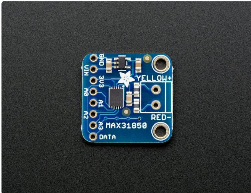
Thermocouples are very sensitive, requiring a good amplifier with a cold-compensation reference. So far we've carried the very nice MAX31855 which is an SPI interface thermocouple amplifier. The '855 is great but if you have a lot of thermocouples to measure it isn't terribly easy to use. That's why we are also carrying the new '850 model from Maxim - it's a "1-Wire" thermocouple amp which can have any number of breakouts on a single shared I/O line.
