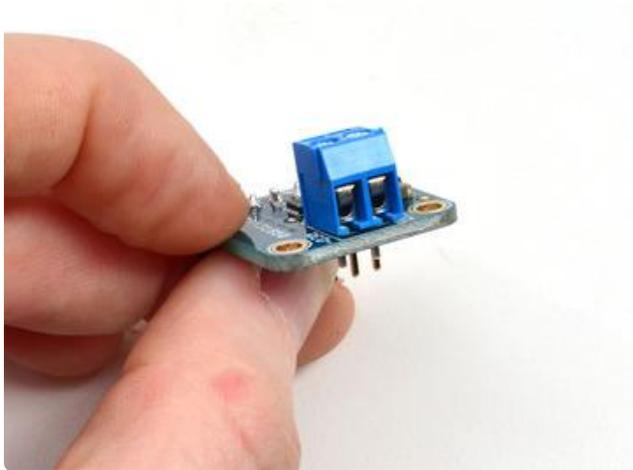
Now you can do the terminal block, this is what you'll use to attach the thermocouple since you cannot solder to thermocouples
