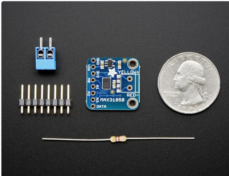
Comes with a 2 pin terminal block (for connecting to the thermocouple), 4.7K data line pullup resistor, and pin header (to plug into any breadboard or perfboard). [Goes great with our 1m K-type thermocouple \(http://adafru.it/270\)](http://adafru.it/270). Not for use with any other kind of thermocouple, K type only!
