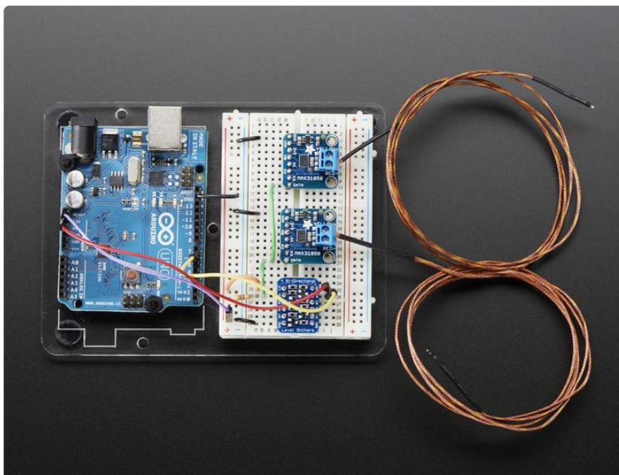
The MAX31850K does everything for you, and can be easily interfaced with any microcontroller that has 1-Wire support. This breakout board has the chip itself, a 3.3V regulator with 10uF bypass capacitors all assembled and tested. This board can be used with 'parasitic power' - where the power is on the data line - or with 'local power' where the power for the converter comes in on the Vin Pin.
