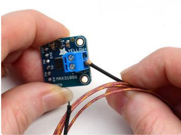
Insert the thermocouple wires and tighten down the clamps with a small Phillips or flat screwdriver
