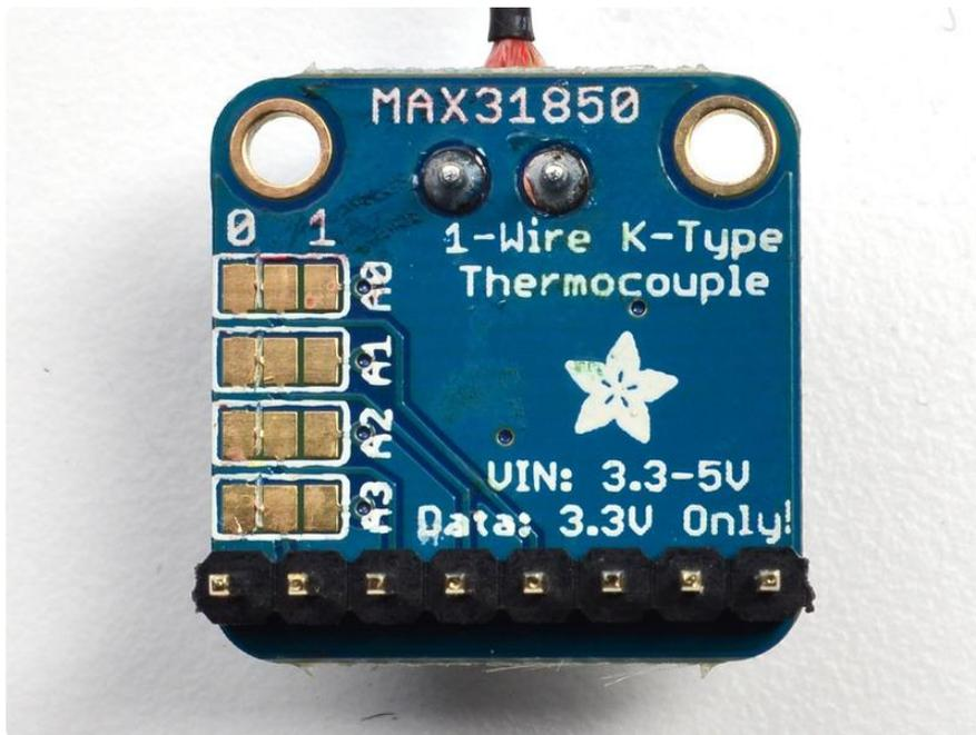
. You can solder the jumpers on the back but we'll be showing wiring with colored wires. In this case, we connect A2 to 3V and the rest to ground, That will make a binary address of 0100 = 0x4
