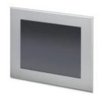
Touch panel with 30.7 cm/12.1" TFT-Display (Analog resistive (polyester)), 800 x 600 Pixel (SVGA), 262144 colors, ARM® Cortex®-A8, 800 MHz, 2x USB host 2.0, 1 x Ethernet (10/100 Mbps), RJ45, Windows® Embedded Compact 7 and User software: IniNet Browser. (Bus system: without)
