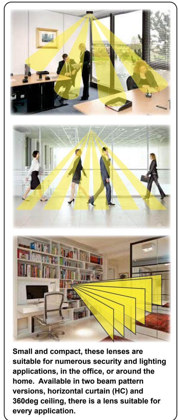
Small and compact, these lenses are suitable for numerous security and lighting applications, in the office, or around the home. Available in two beam pattern versions, horizontal curtain (HC) and 360deg ceiling, there is a lens suitable for every application.
