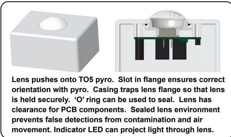
Lens pushes onto TO5 pyro. Slot in flange ensures correct orientation with pyro. Casing traps lens flange so that lens is held securely. 'O' ring can be used to seal. Lens has clearance for PCB components. Sealed lens environment prevents false detections from contamination and air movement. Indicator LED can project light through lens.
