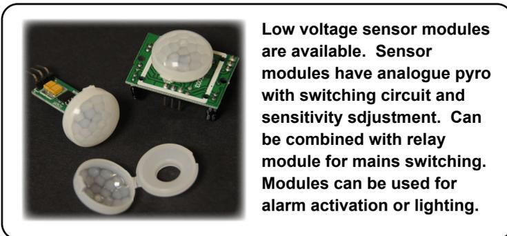
Low voltage sensor modules are available. Sensor modules have analogue pyro with switching circuit and sensitivity adjustment. Can be combined with relay module for mains switching. Modules can be used for alarm activation or lighting.
