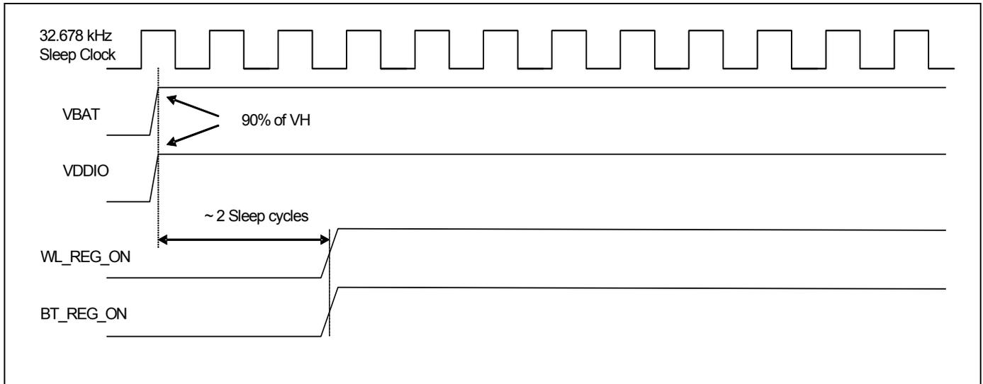
**Figure 39. WLAN = OFF, Bluetooth = OFF**
