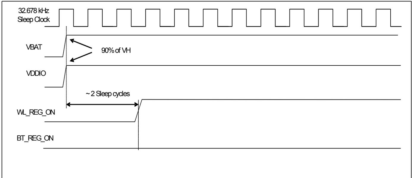
**Figure 41. WLAN = OFF, Bluetooth = ON**
