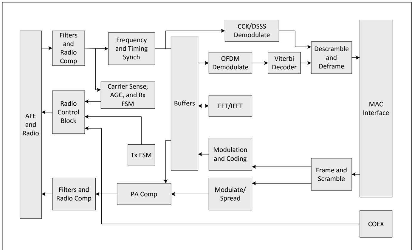
The PHY is capable of fully calibrating the RF front-end to extract the highest performance. On power-up, the PHY performs a full calibration suite to correct for IQ mismatch and local oscillator leakage. The PHY also performs periodic calibration to compensate for any temperature related drift, thus maintaining high-performance over time. A closed-loop transmit control algorithm maintains the output power at its required level and can control TX power on a per-packet basis.
