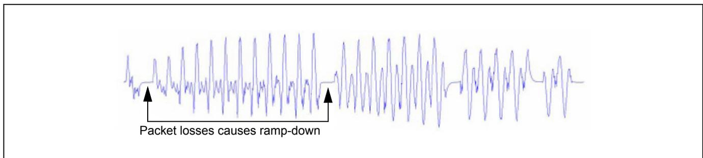
**Figure 21. CVSD Decoder Output Waveform After Applying PLC**
