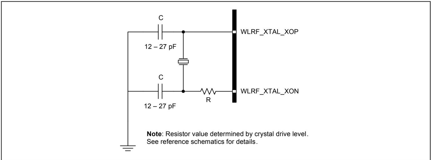
The CYW43438 uses a fractional-N synthesizer to generate the radio frequencies, clocks, and data/packet timing so that it can operate using numerous frequency references. The frequency reference can be an external source such as a TCXO or a crystal interfaced directly to the CYW43438.
