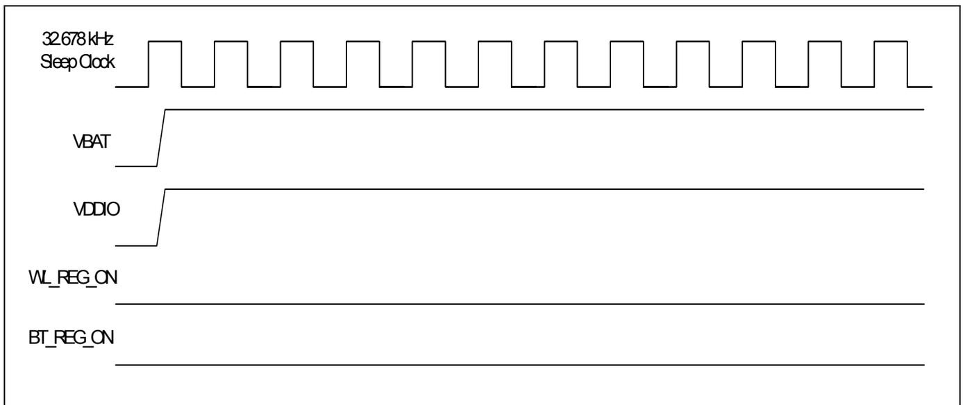
**Figure 40. WLAN = ON, Bluetooth = OFF**
