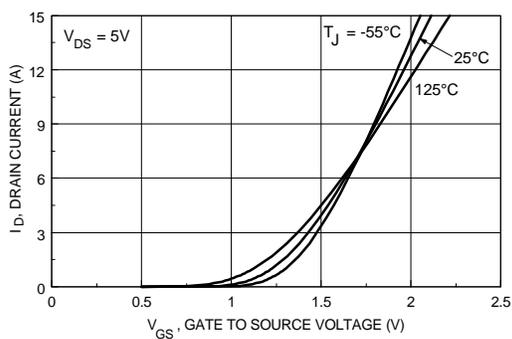
Figure 5. Transfer Characteristics.
