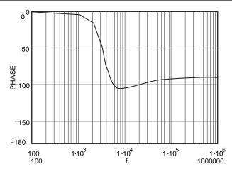
Figure 5. Phase Curve for G(s)
