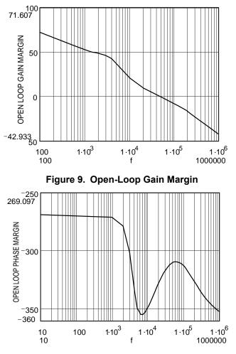
Figure 10. Open-Loop Phase Margin
