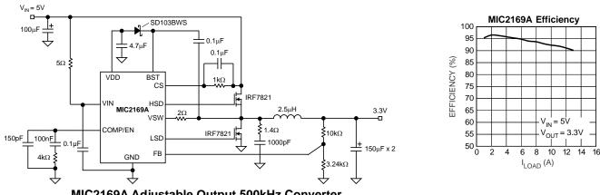
MIC2169A Adjustable Output 500kHz Converter
