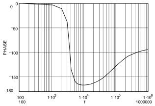
Figure 6. The Phase Curve with ESR =  $0.002\Omega$
