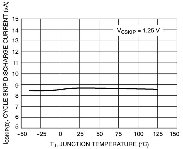
**Figure 19. Cycle Skip Discharge Current vs. Junction Temperature**
