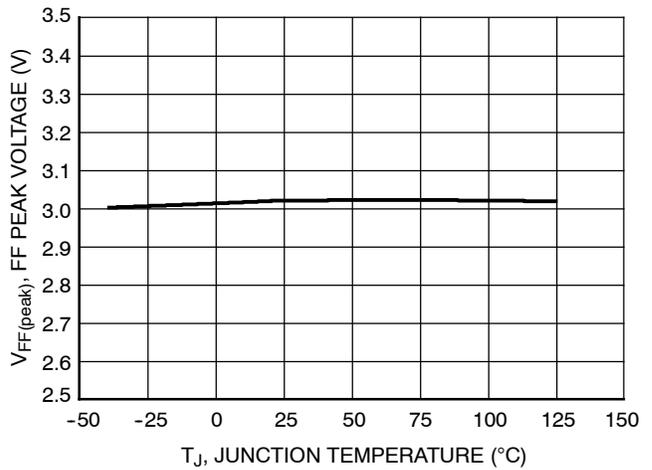
**Figure 14. Feedforward Peak Voltage vs. Junction Temperature**
