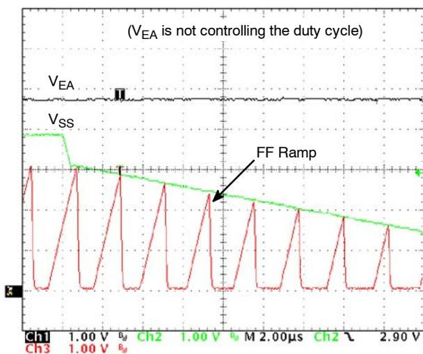
**Figure 36. Soft-Stop Behavior After Soft-Start is Complete and V<sub>EA</sub> is Open.**
