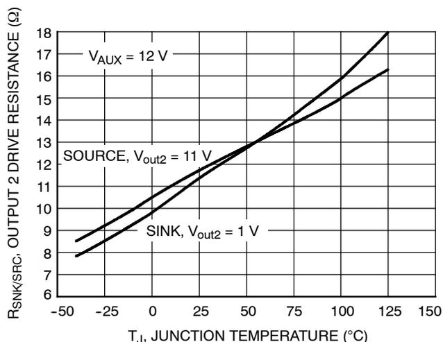
**Figure 31. Output 2 Drive Resistance vs. Junction Temperature**
