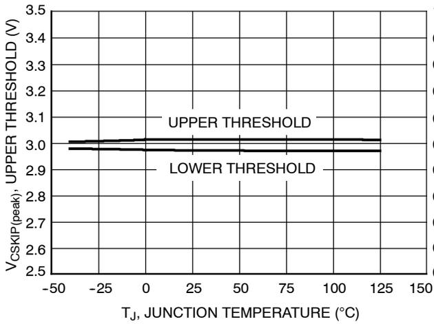
**Figure 20. Cycle Skip Voltage Thresholds vs. Junction Temperature**
