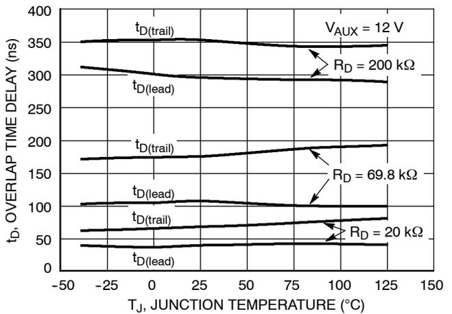
**Figure 29. Overlap Time Delay vs. Junction Temperature**
