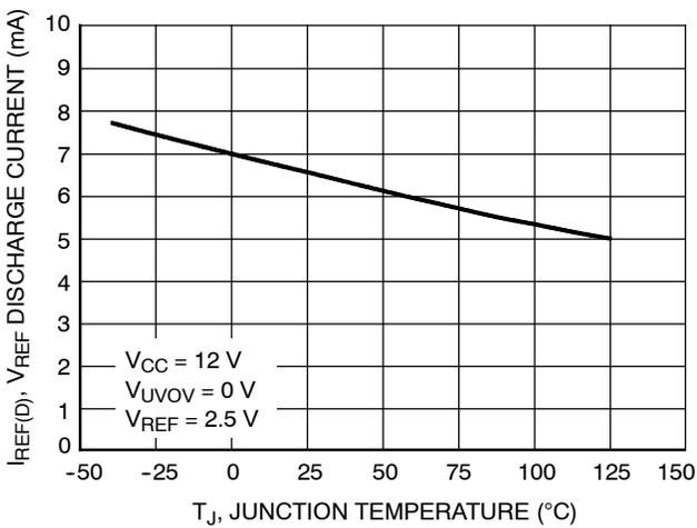
**Figure 22.  $V_{REF}$  Discharge Current vs. Junction Temperature**
