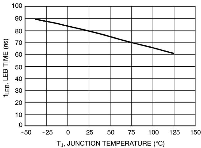
**Figure 17. Leading Edge Blanking Time vs. Junction Temperature**
