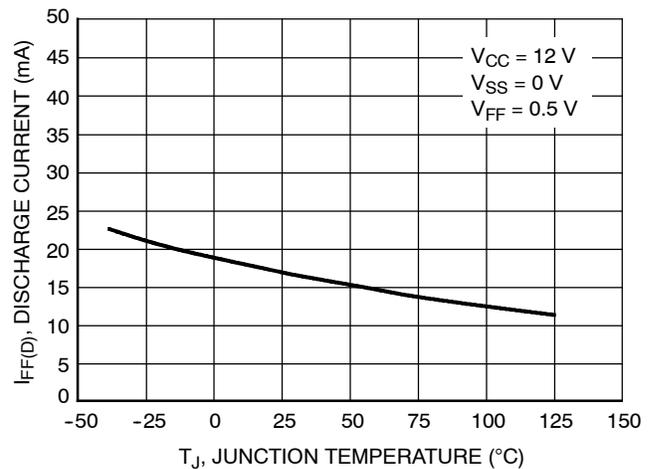
**Figure 12. FF Discharge Current vs. Junction Temperature**
