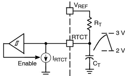
Figure 48. Oscillator Configuration
