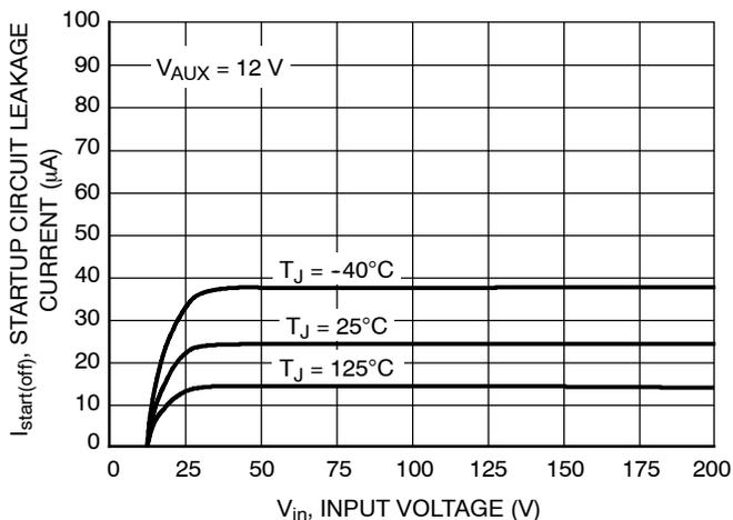
**Figure 6. Startup Circuit Leakage Current vs. Input Voltage**
