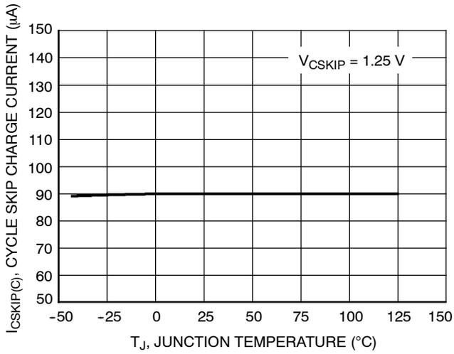
**Figure 18. Cycle Skip Charge Current vs. Junction Temperature**
