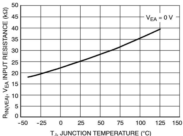
**Figure 32.  $V_{EA}$  Input Resistance vs. Junction Temperature**
