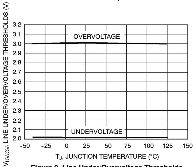
**Figure 9. Line Under/Overvoltage Thresholds vs. Junction Temperature**
