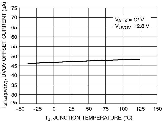
**Figure 11. UV OV Offset Current vs. Junction Temperature**
