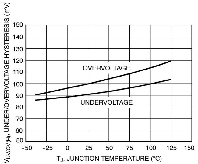
**Figure 10. Line Under/Overvoltage Hysteresis vs. Junction Temperature**
