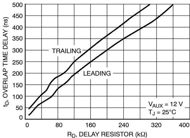
**Figure 28. Overlap Time Delay vs. Delay Resistor**
