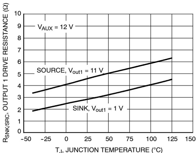
**Figure 30. Output 1 Drive Resistance vs. Junction Temperature**
