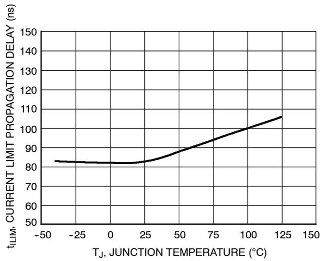
**Figure 16. Current Limit Propagation Delay vs. Junction Temperature**
