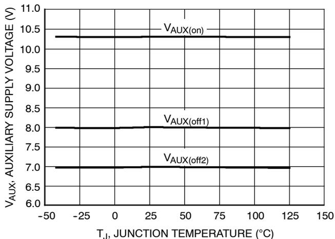
**Figure 3. Auxiliary Supply Voltage Thresholds vs. Junction Temperature**
