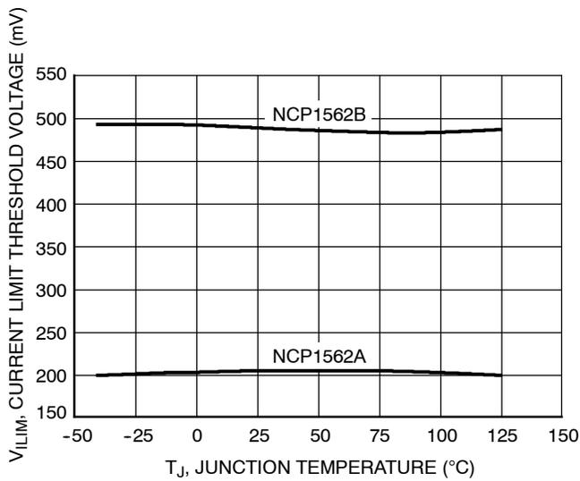
**Figure 15. Current Limit Threshold Voltage vs. Junction Temperature**
