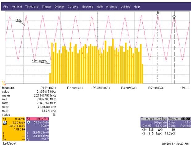
Spread spectrum is automatically turned off when there is a short to GND or an open circuit on either the RMOD pin or the RDEPTH pin. Please be sure that the ROSC pin is an open circuit when using spread spectrum.
