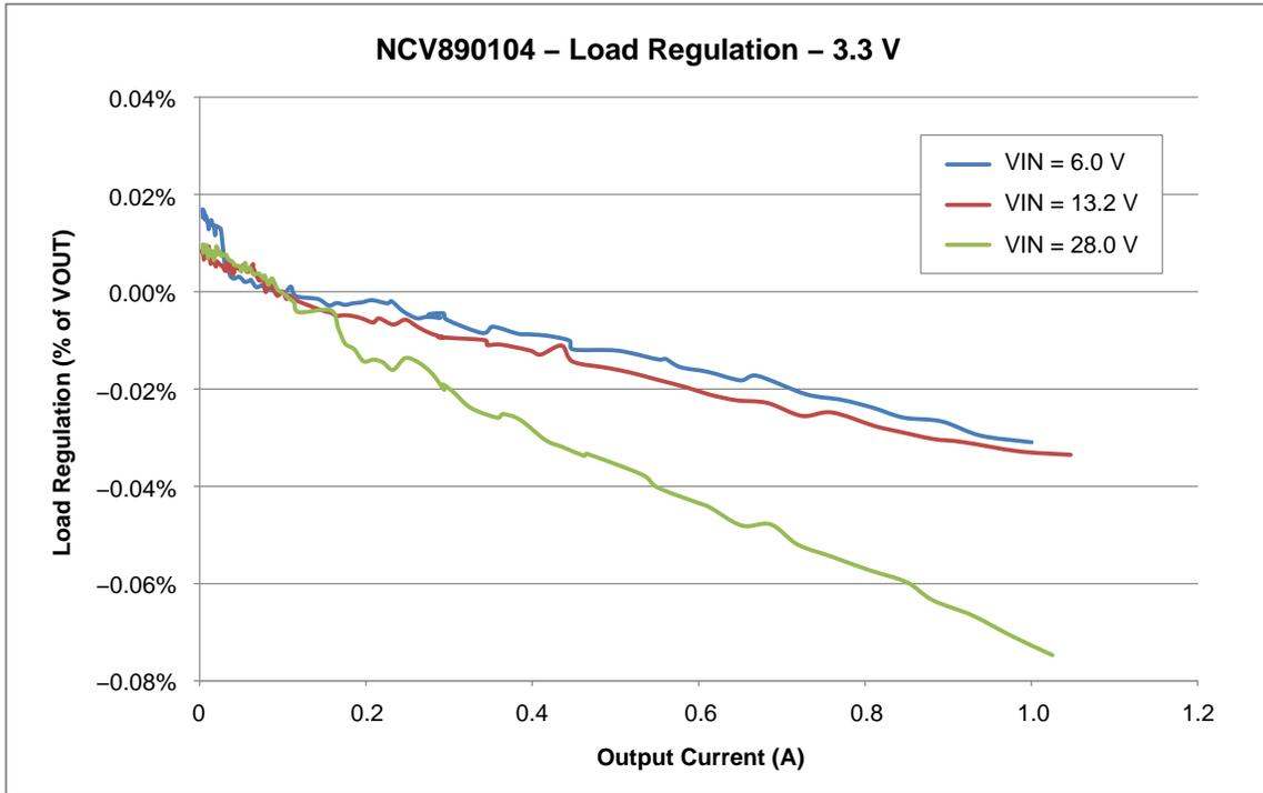
Figure 12. Load Regulation with a 3.3 V Output
