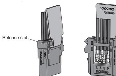
(4) Move the jig as follows and release operating lever at once.
