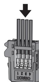
(3) Insert operation jig into lock release slot.
