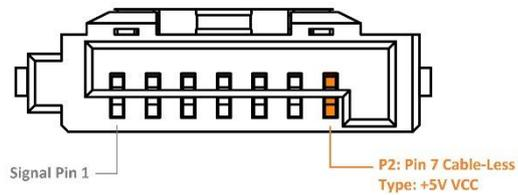
Table 3-3 Signal/Power Segment (Pin 7 Cable-less)
