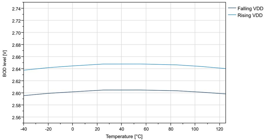
**Figure 38-54. BOD Threshold vs. Temperature (Level 4.3V)**
