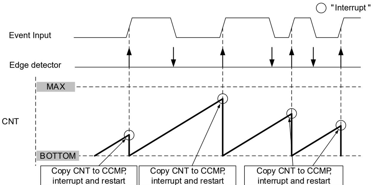
**21.3.3.1.5 Input Capture Pulse-Width Measurement Mode**
