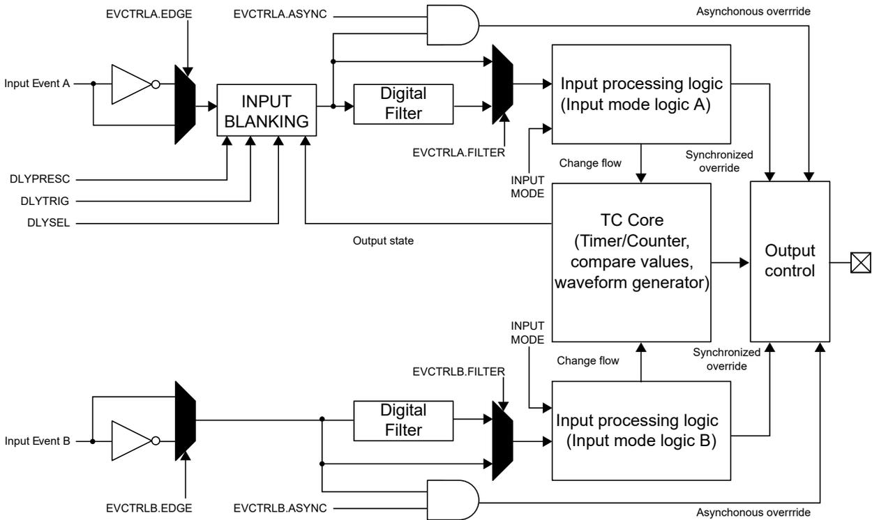
There is a delay of 2-3 clock cycles on the TCD synchronizer clock between receiving the input event, processing it, and overriding the outputs. If using the asynchronous event detection, the outputs will override instantly outside the input processing.
