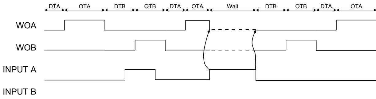
If Input mode 1 is used on input B, an event will only have an effect if the TCD is in Dead-time B or On-time B, and it will only affect the output WOB. When the event is done, the TCD counter starts at Dead-time A.
