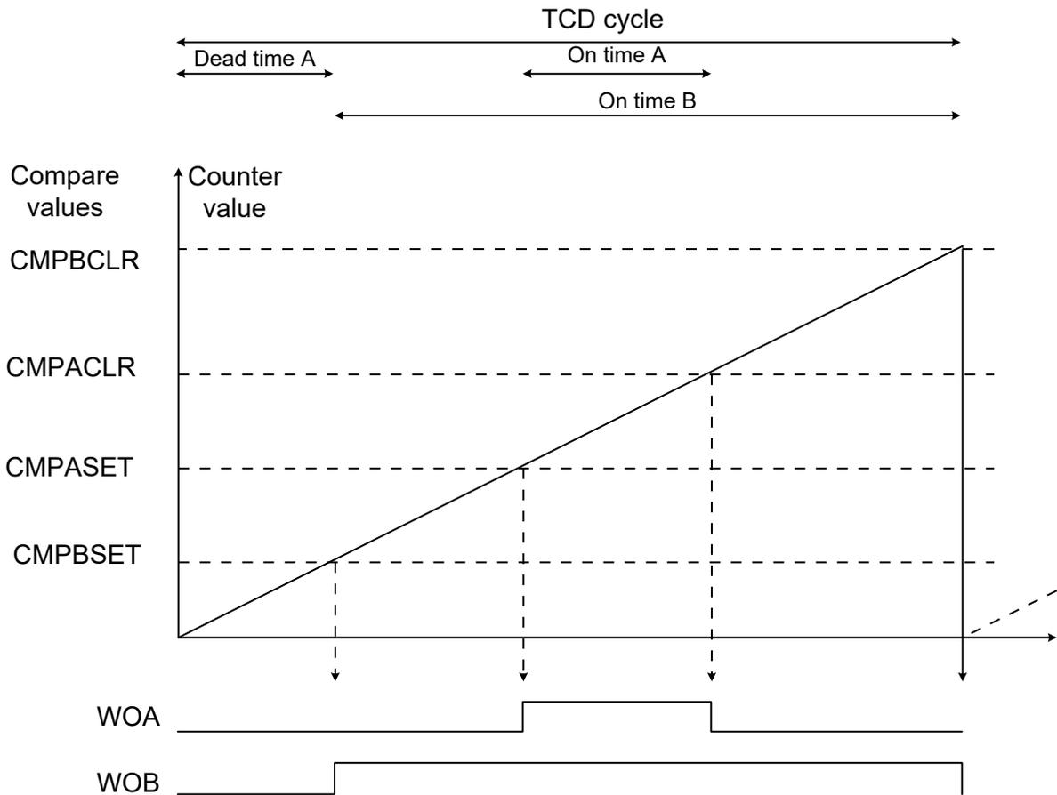
If any of the other compare values are bigger than CMPBCLR it will never be triggered when running in One Ramp mode, and if the CMPACLR is smaller than the CMPASET value, the clear value will not have any effect.
