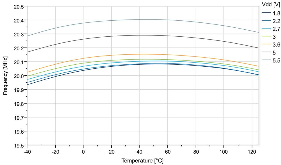
**Figure 38-76. OSC20M Internal Oscillator: Frequency vs. V<sub>DD</sub>**
