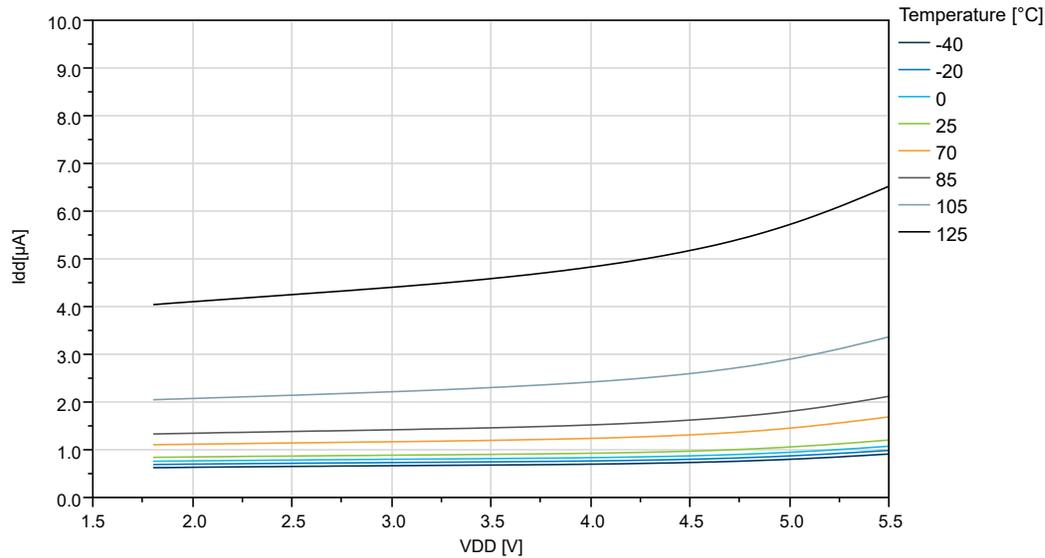
**Figure 38-13. ATtiny1617 Standby Mode Supply Current vs.  $V_{DD}$  (RTC Running with Internal OSCULP32K)**
