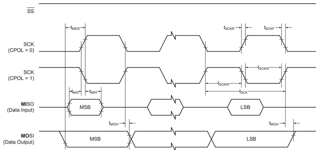
**Table 37-19. USART in SPI Master Mode - Timing Characteristics**
