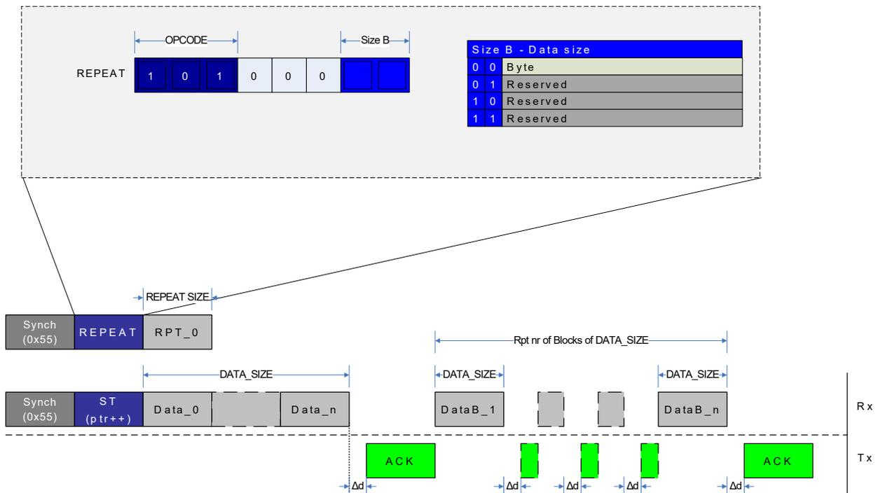
The figure above gives an example of repeat operation with an ST instruction using pointer post-increment operation. After the REPEAT instruction is sent with RPT\_0 = n, the first ST instruction is issued with SYNCH and Instruction frame, while the next n ST instructions are executed by only sending in data bytes according to the ST operand DATA\_SIZE, and maintaining the Acknowledge (ACK) handshake protocol.
