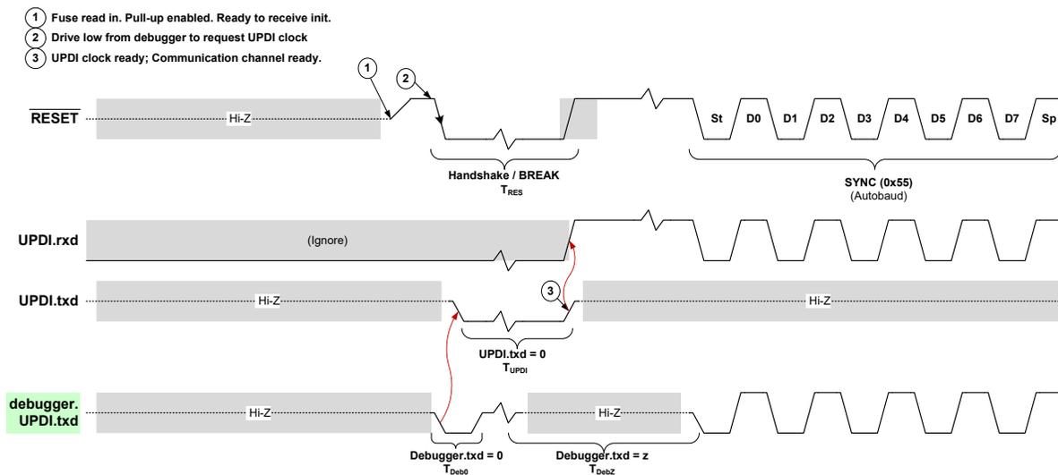
When the pull-up is detected, the debugger initiates the enable sequence by driving the line low for a duration of  $T_{Deb0}$  to ensure that the line is released from the debugger before the UPDI enable sequence is done.
