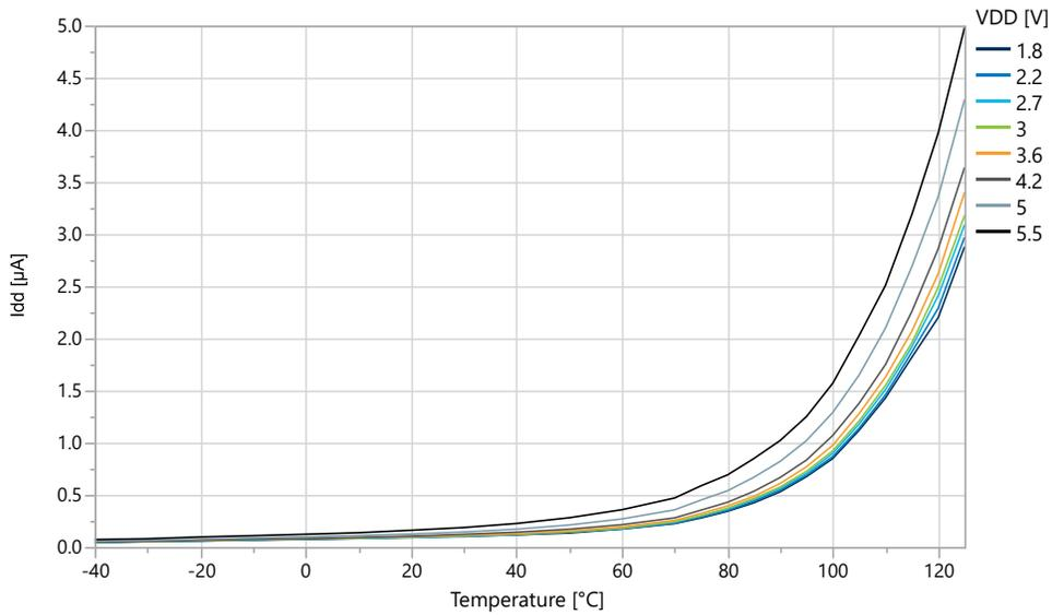
**Figure 38-11. ATtiny1617 Power-Down Mode Supply Current vs.  $V_{DD}$  (all functions disabled)**
