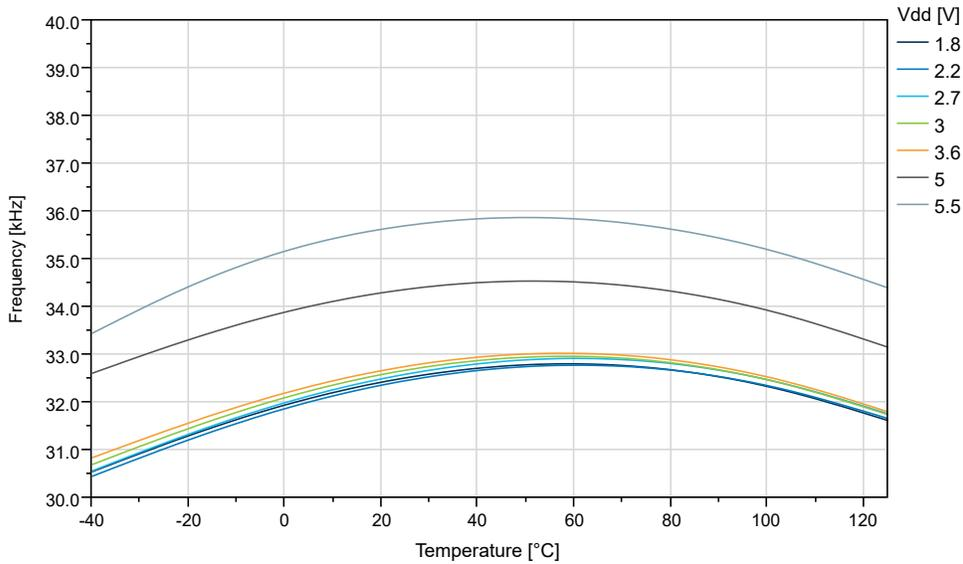
**Figure 38-78. OSCULP32K Internal Oscillator Frequency vs. V<sub>DD</sub>**
