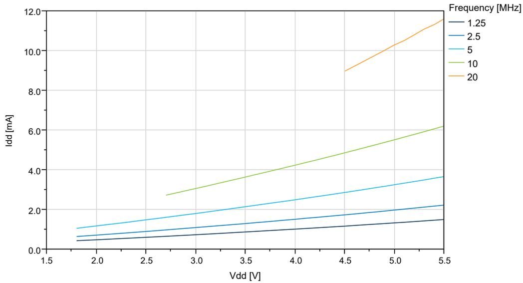
**Figure 38-5. ATtiny1617 Active Supply Current vs.  $V_{DD}$  (f=32 KHz OSCULP32K)**
