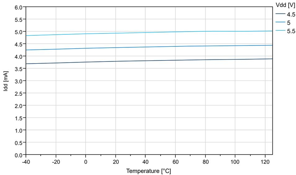
**Figure 38-9. ATtiny1617 Idle Supply Current vs.  $V_{DD}$  (f=32 KHz OSCULP32K)**
