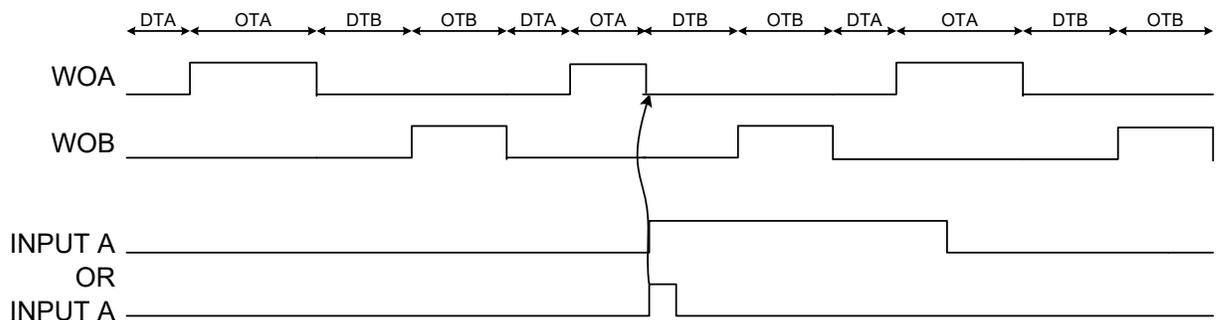
If Input mode 8 is used on input B and a positive input event occurs while in On-time B, the TCD counter jumps to Dead-time A.
