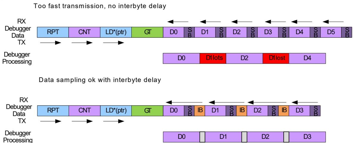
GT denotes the Guard Time insertion, SB is for Stop bit and IB is the inserted interbyte delay. The rest of the frames are data and instructions.
