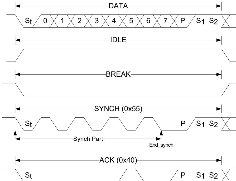
**Data Frame** Data frame consists of one Start bit (always low), eight data bits, one parity bit (even parity), and two Stop bits (always high). If the Start bit, parity bit, or Stop bits have an incorrect value, an error will be detected and signaled by the UPDI. The parity bit-check in the UPDI can be disabled by writing the PARD bit in UPDI.CTRLA, in which case the parity generation from the debugger can be ignored.
