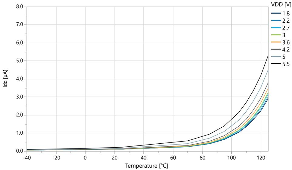
Figure 38-29. ATtiny3217 Power-Down Mode Supply Current vs.  $V_{DD}$  (all functions disabled)
