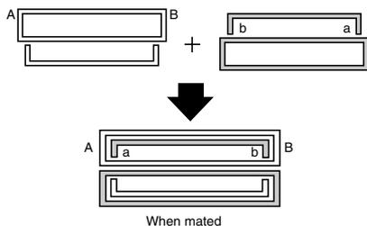
**3. Ideal for portable devices, the bellows-type contacts provide a strong resistance against falling, impacts, and forced insertions and removals.**
