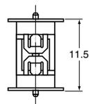
• Mated height 11.5mm type (Socket and Header)
