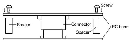
When connecting PC boards, take appropriate measures to prevent the connector from coming off.
