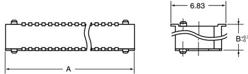
Mated height 11.5mm type (Socket and Header)
