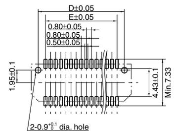
Note: The 13 mm mated height (20 to 80 pin contacts) terminal flatness is 0.1 mm.
