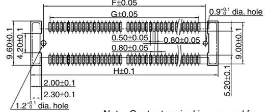
Note: Center terminal is removed for 80 and 100 pin contact type
