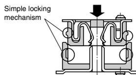
The simple lock mechanism is not featured on the 11.5 mm version. However, proper contact and resistance against vibrations and shocks are both ensured by the long mating length.
