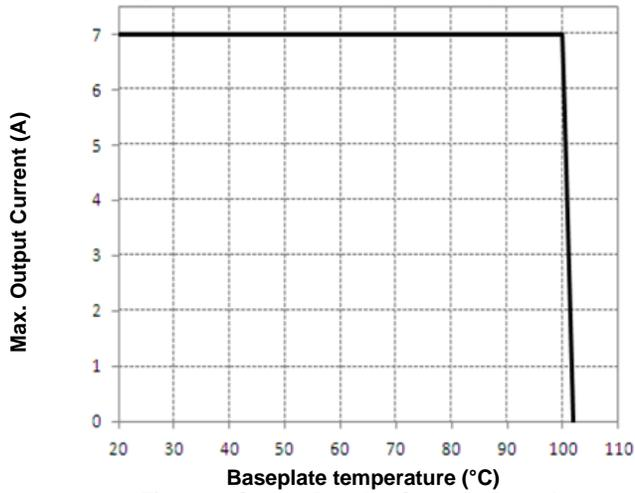
**Figure 9.** Current Derating Curve for Baseplate
