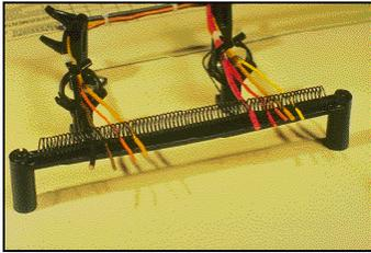
Consists of harness board springs and spring holders to hold wire ends taut. When harness is removed from board, wires simply pull from spring.
