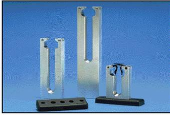
Used to hold and support the THM1SC Harness Mount. The mount is elevated from the harness board so that a cable tie can be installed by Panduit's automatic cable tie installation tools. The mount is pushed into the top of the fixture prior to assembly and pulled out of the fixture when the harness is complete.
