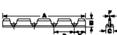
Designed to hold FS156 Fanning Strip securely in place while wires are inserted into fanning strip.
