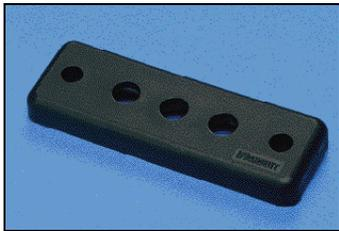
Used with the Harness Board Standoff Post or the Harness Mount Fixture when mounting holes can not be drilled into the harness board. A bolt is inserted from the back side of the adapter and then is turned right side up. The adapter is now ready to be secured to the harness board by using self tapping screws.
