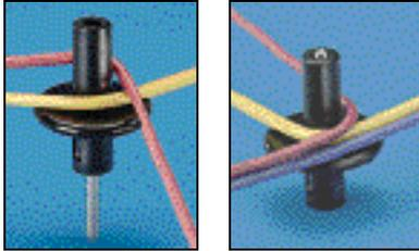
The "up" position allows forming of harness and cable tie installation
