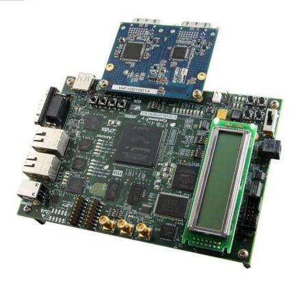
The Cyclone V E Video Development System is an ideal video processing platform for high-performance, cost-effective video applications. The Cyclone® V E Development Kit offers a comprehensive general purpose development platform for many markets and applications. With multiple banks of DDR3 and LPDDR2 memory, this kit provides the ideal low-cost platform for high-bandwidth video processing. Additional features include an LCD character display, LEDs, user switches, USB and RJ-45 connectors.
