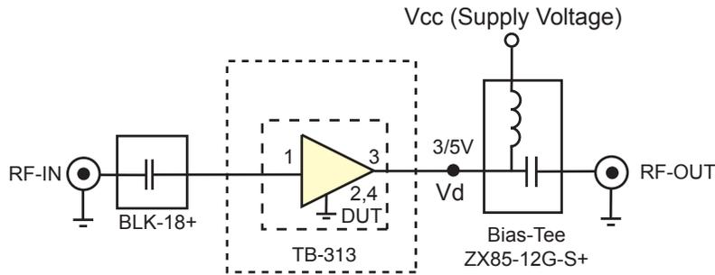
**Fig 1.** Block Diagram of Test Circuit used for characterization. (DUT tested on Mini-Circuits Characterization test board TB-313) Gain, Return loss, Output power at 1dB compression (P1 dB) , output IP3 (OIP3) and noise figure measured using Agilent’s N5242A PNA-X microwave network analyzer.
