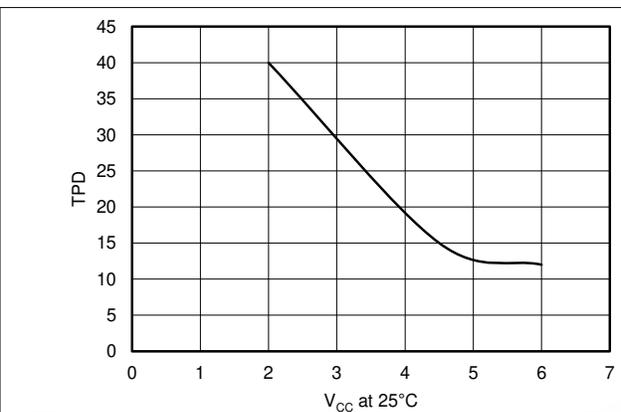
Figure 6-2. TPD vs  $V_{CC}$  at  $25^\circ\text{C}$
