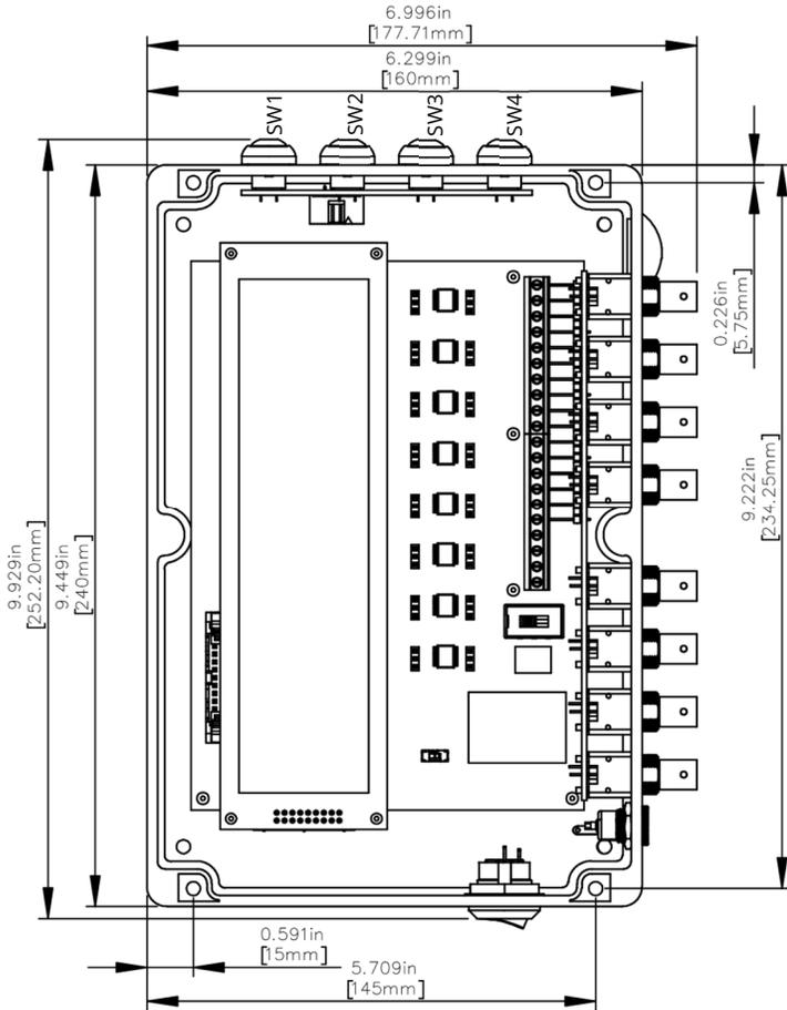
Use the following hole pattern if using the mounting screws provided with the Sensor Interface System enclosure:
