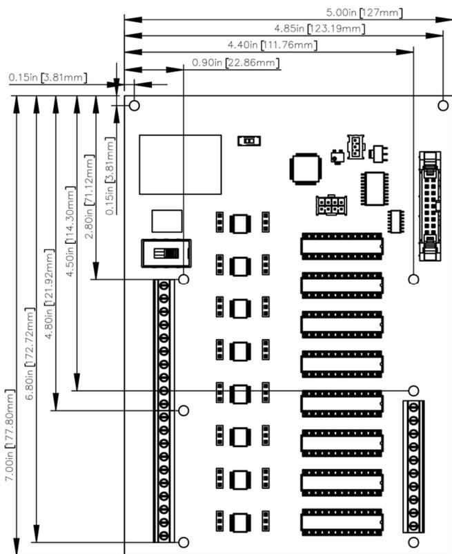
Use the provided spacers and screws when installing the *WaterFeature8*. If other mounting methods are preferred, consider that the board is 0.063" (1.6 mm) thick when selecting mounting devices.
