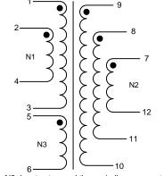
N1, N2 denotes two and three windings connected in parallel. Terminals 1+2, 3+4, 7+8+9 and 10+11+12 must be tied as solder bridging is allowed.
