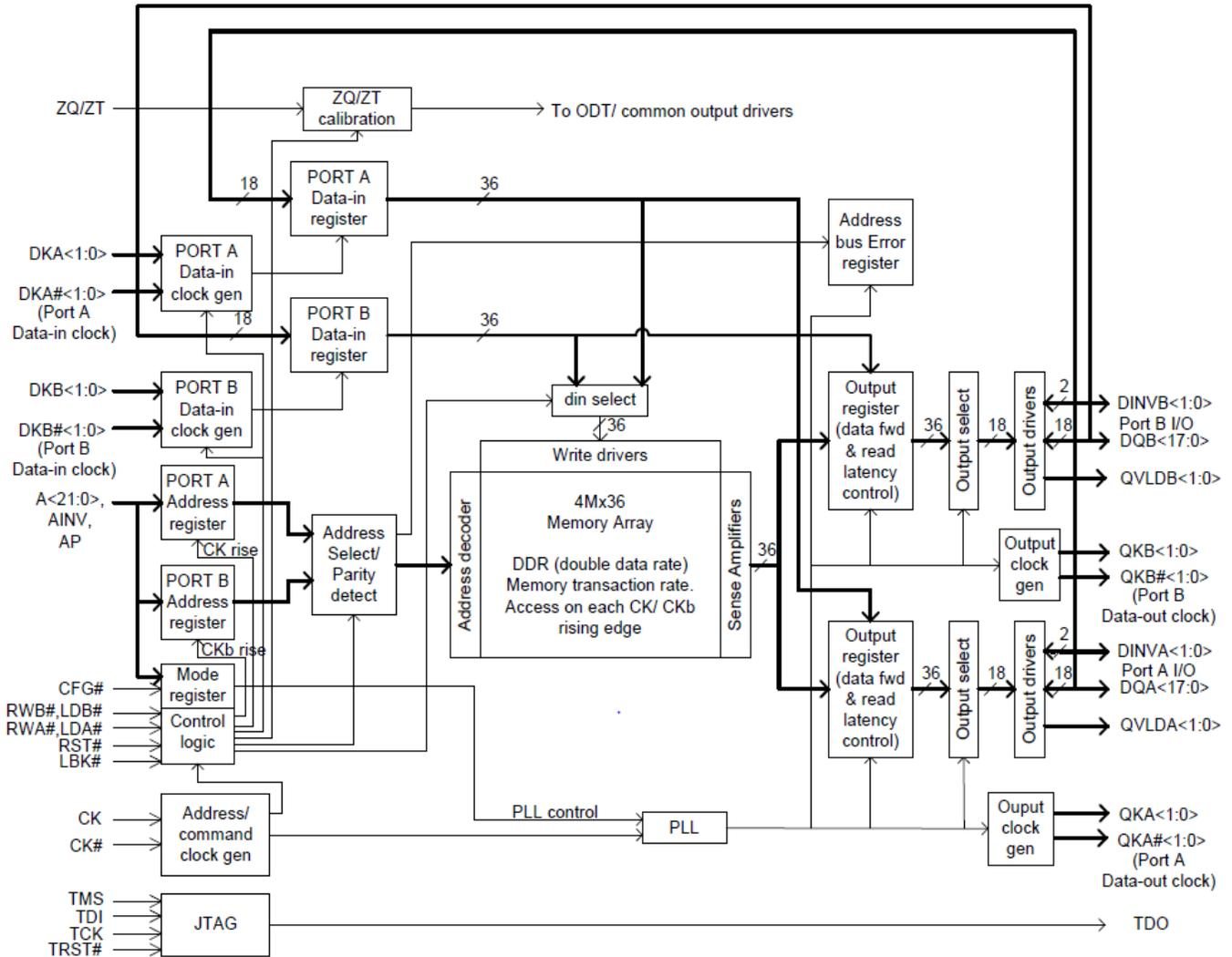
Logic Block Diagram – CY7C4141KV13
