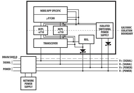
Figure 19. Isolated node powered by the network
