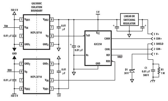
Figure 22. Recommended DeviceNet application circuit
