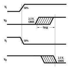
Figure 15. Propagation delay skew waveform
