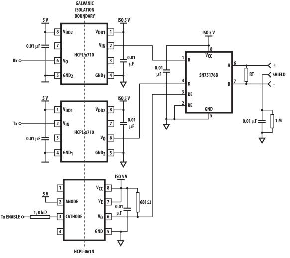
Figure 24. Recommended PROFIBUS application circuit
