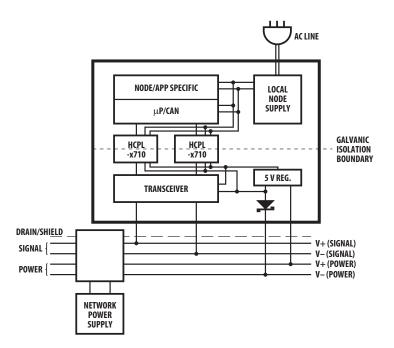
Figure 18. Typical DeviceNet node.
