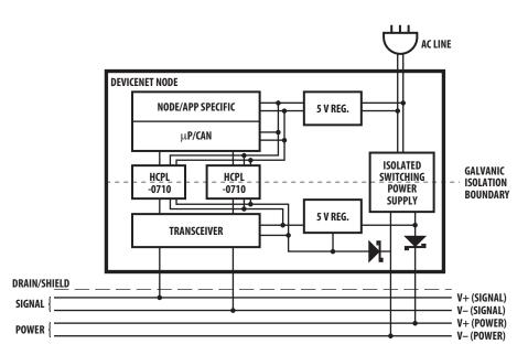
Figure 21. Isolated node providing power to the network
