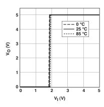
Figure 1. Typical output voltage vs. input voltage
