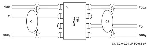
Figure 13. Recommended Printed Circuit Board layout.
