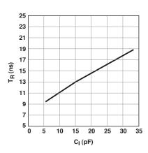
Figure 9. Typical rise time vs. load capacitance
