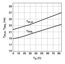
Figure 3. Typical propagation delays vs. temperature
