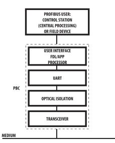
Figure 23. PROFIBUS Controller (PBC)
