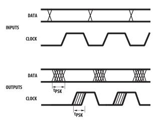
Figure 16. Parallel data transmission example
