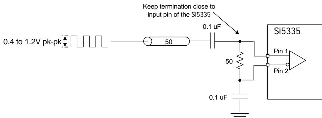
Figure 12. Single-Ended Input Signal with 50  $\Omega$  Termination
