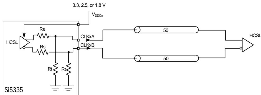
Figure 20. Interfacing the Si5335 to an HCSL Receiver
