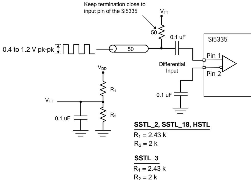
**Figure 11. Single-Ended SSTL/HSTL Input Clocks to the Si5335**
