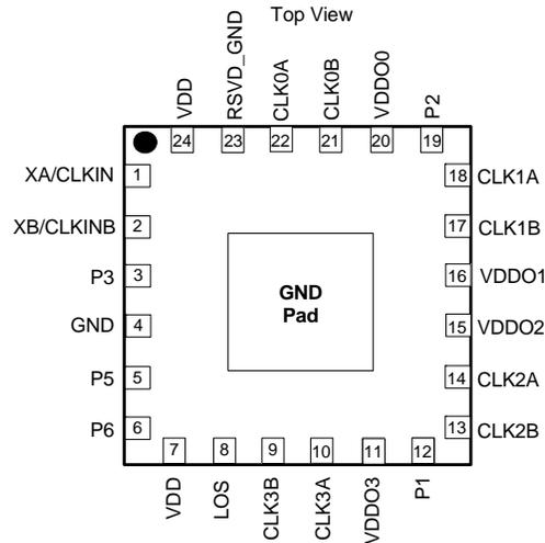
**Note:** Center pad must be tied to GND for normal operation.
