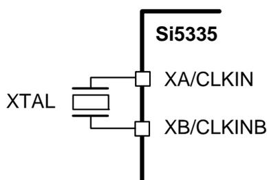
Figure 4. Connecting an XTAL to the Si5335
