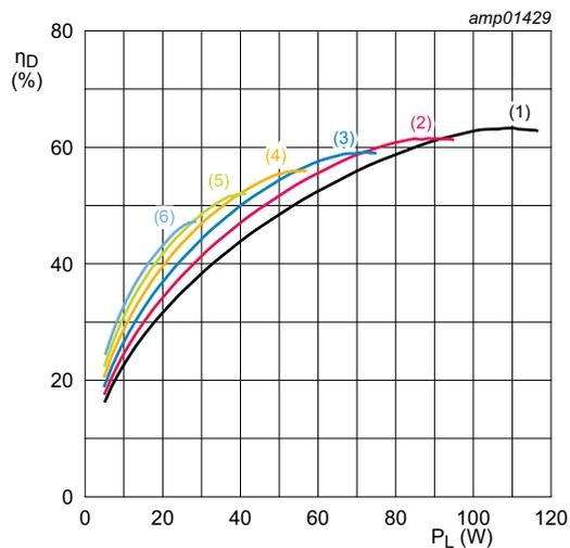
$I_{Dq} = 30 \text{ mA}; f = 1400 \text{ MHz}; t_p = 100 \text{ }\mu\text{s}; \delta = 20 \text{ \%}.$
