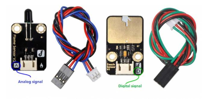
• This is DFRobot's **Gravity Interface**. Digital and analog connections are easy to recognize and support most of DFRobot's I/O expansion shields and modules. Search **"Gravity"** in the DFRobot store to find compatible modules.
