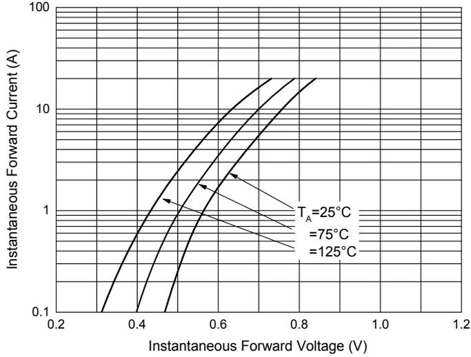
Fig. 4 - MBR30150FCTH Typical Instantaneous Forward Characteristics
