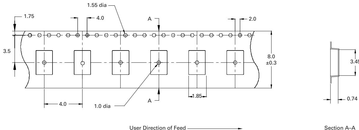
Supplied in tape and reel packaging, 2500 parts per 7.0" diameter reel (EIA-481 compliant)
