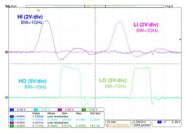
Figure 8-2. Input and Output Pulse Width
