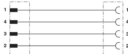
Contact assignment of M8 plugs / M12 sockets
