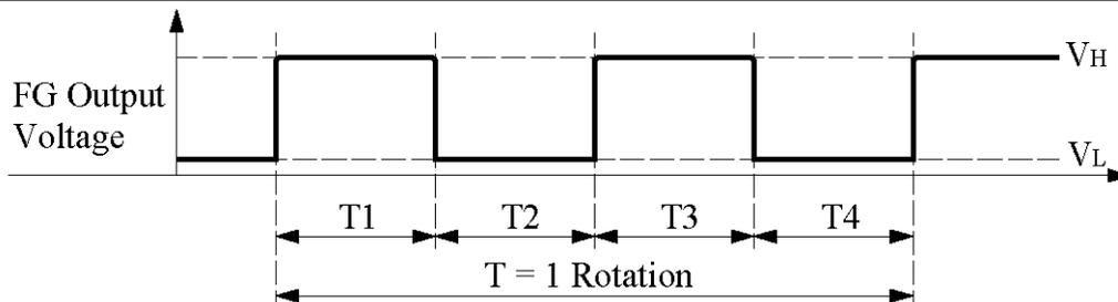
$$T = T_1 + T_2 + T_3 + T_4 = 1 \text{ Rotation}$$
